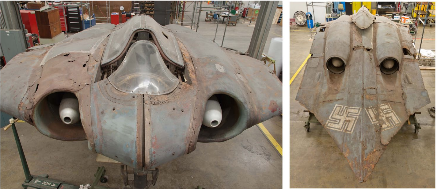
Fig. 1. The Horten Ho 229V3 (A19600324000) in the NASM collection. Views of the aircraft from the front and back. Height: 9', Length: 25', Wingspan: 55' (wings not attached in photos). Images Ben Sullivan 2013.
