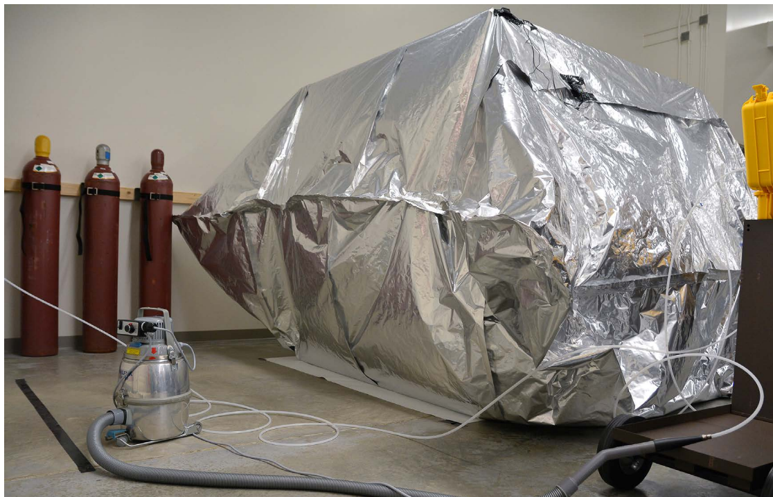
Fig. 1. Example of a large scale anoxic envelope used in the treatment of museum objects. Photo by Eugenie Milroy
