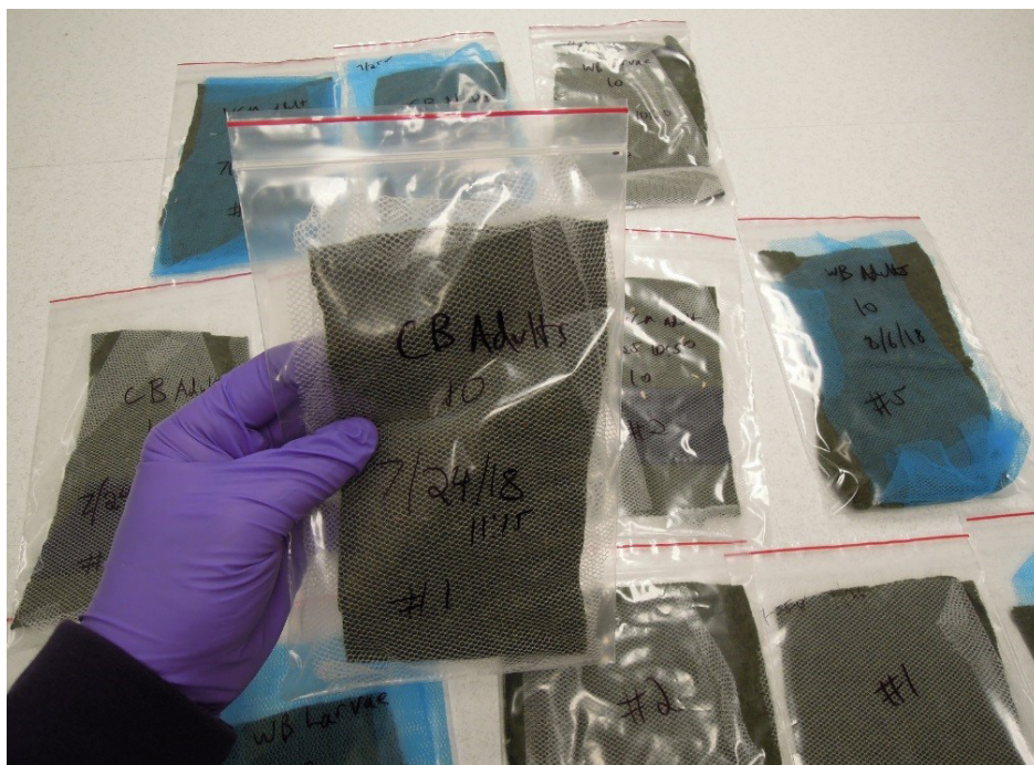
Figure 1. Entomological testing, where a food source was wrapped in LLIN, sealed with the pest species, and then monitored for mortality results over time. Courtesy of Pat Kelley, Insects Ltd., 2018.
