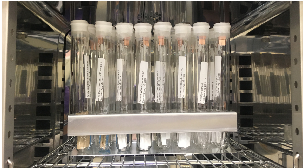
The MWG Testing & Standards committee is testing materials using a round-robin method at several institutions. The samples in test tubes (above) and lead acetate test papers (below right) were tested at National Museum of the American Indian, Smithsonian Institution. Courtesy Lisa Imamura.
