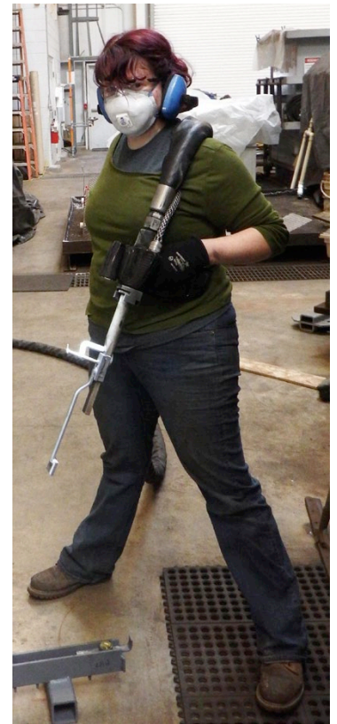
Figure 4 (above). Mariners' staff member Laurie King is seen wearing all of the appropriate PPE for dry ice blasting treatment: ear protection, eye protection, respirator mask, cold protection gloves, long sleeves, trousers, and boots. Image courtesy of The Mariners' Museum and Park.
