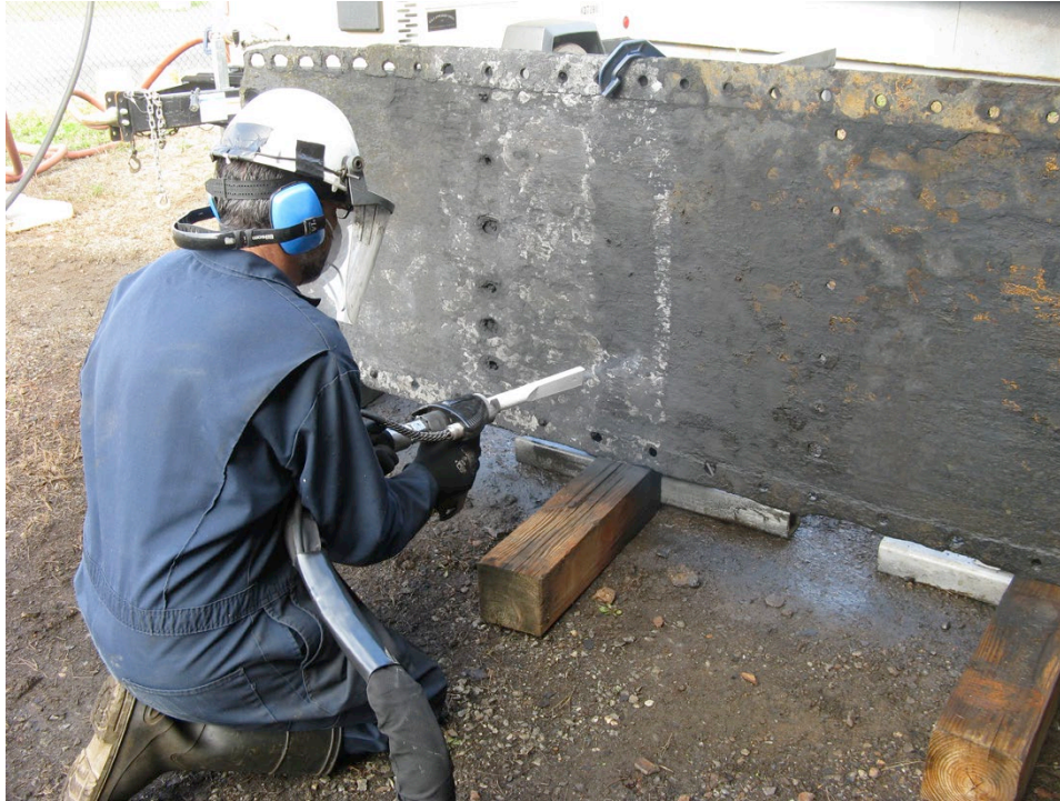
Figure 6. Mariners' staff member Michael Saul is treating an archaeological iron object while wearing all appropriate PPE, including cold protection gloves. Image courtesy of The Mariners' Museum and Park.
