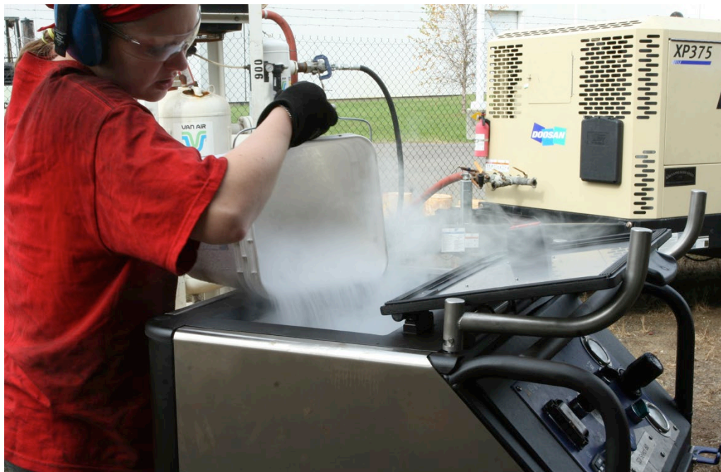
Figure 3. Mariners' staff member Kate Sullivan is seen pouring dry ice pellets into the blasting unit, wearing the appropriate protective equipment. Image courtesy of The Mariners' Museum and Park.
