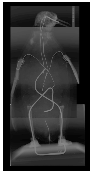
Figure 11. Stitched x-radiograph of the emperor penguin taxidermy mount showing the original mounting system (130kV, 150mAs).
