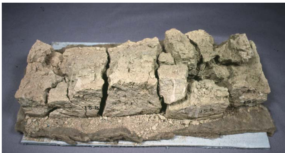
Figure 12. In 1990, one crate was opened and the bricks were removed for examination. The bricks were in a very fragile and fragmentary condition. Consolidation tests were conducted on these bricks to determine which consolidant was most effective. The bricks had also been treated in the field with a cellulose-nitrate based adhesive (“Ambroid”; Loud 1933), and the tests would help determine the compatibility of the modern resin with the aged cellulose-nitrate consolidant. Glazed clay brick, Sin Temple, Khorsabad, Iraq, 722-705 BC, Oriental Institute Museum, OIM A11810.158.
