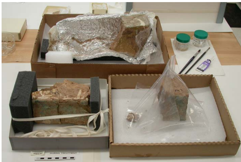
Figure 15. Excess dirt was removed from each brick by both brush-vacuuming and lightly swabbing with 1:1 ethanol:deionized water where necessary. The bricks were then consolidated several times with a 3-5% solution of Acryloid B-72; after each consolidation, the pieces were placed in polyethylene bags to retard solvent evaporation. Glazed bricks, Sin Temple, Khorsabad, Iraq, 722-705 BC, Oriental Institute Museum, OIM A11810.147.
