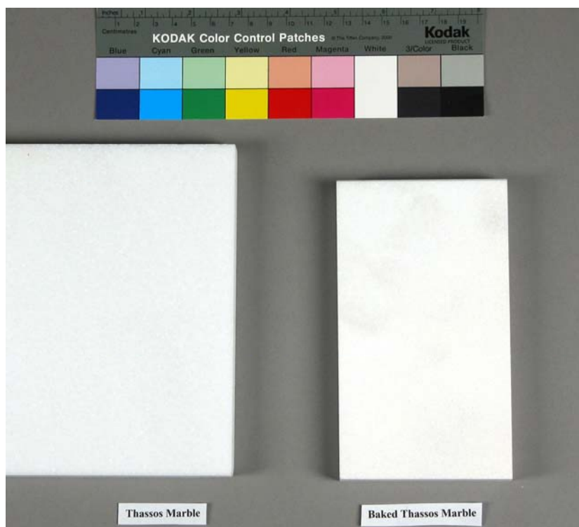
Figure 6. Test using baked Thassos marble.
