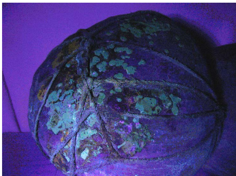
Figure 2. A Tarahumara pot with an ethnographic repair. Under UV, it is clear that there are two adhesives: a green-fluorescing adhesive over an orange-fluorescing adhesive. The color of the fluorescence determines the next testing step. Photograph by Margaret Kipling.
