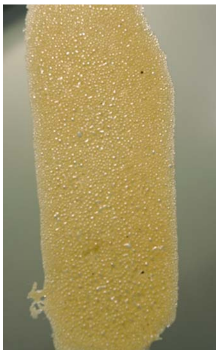
Figure 9. Unsuccessful film with air bubbles
