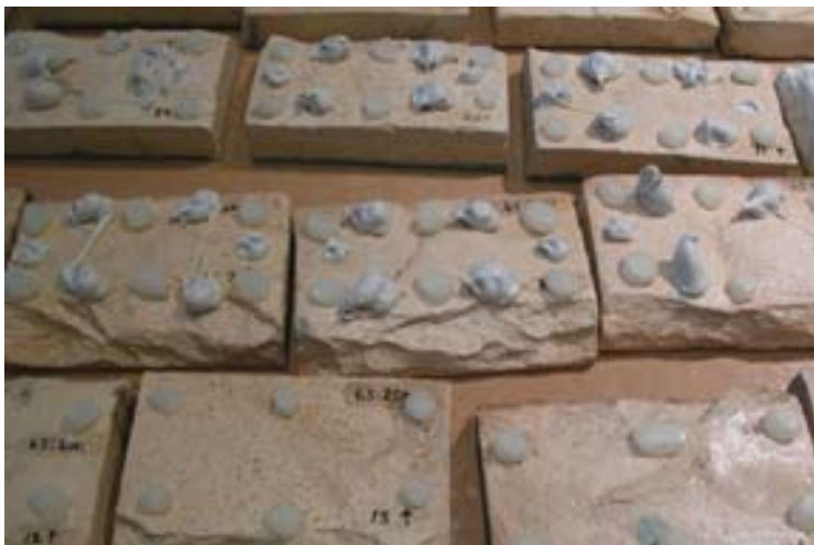
Figure 9. Epoxy piped between the wax stilts.
