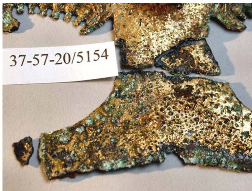
Fig. 5. Delamination caused by Alvar coating (PMAE# 37-57-20/ 5154).
