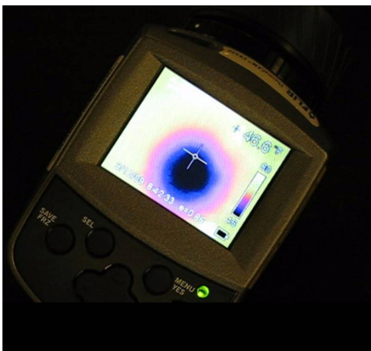
Fig. 1. The display screen of the FLIR unit showing the low temperature value of 46.6°F. The black spot on the screen is the CO 2 snow jet in direct contact with the instrument's lens. (Photograph by Shockey)
