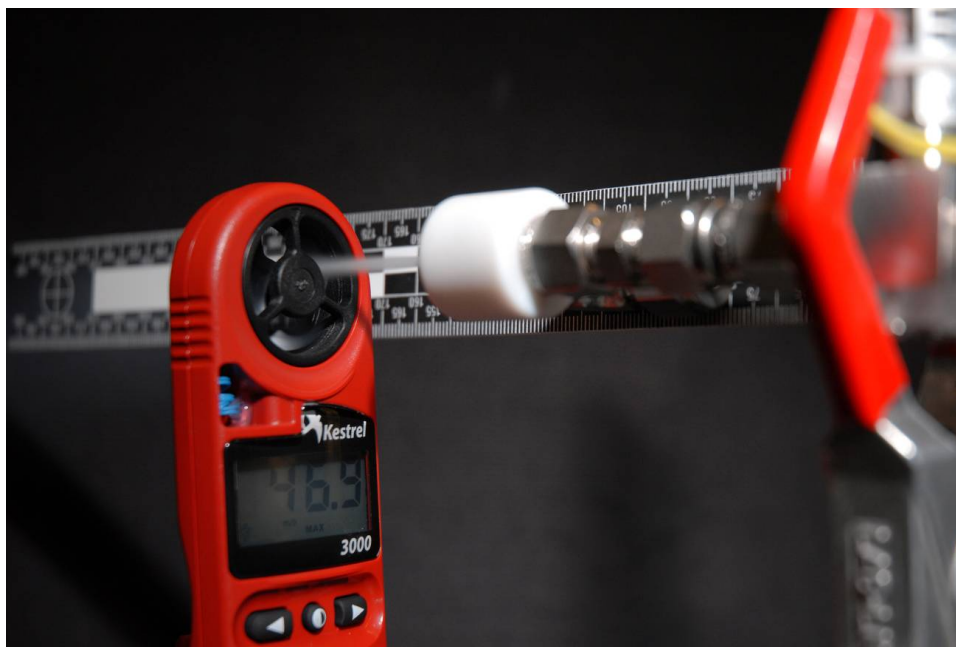
Fig. 3. Velocity testing in the conservation lab. The white CO 2 snow jet can be seen between the end of the nozzle and the entrance of the meter. (Photograph by Shockey)
