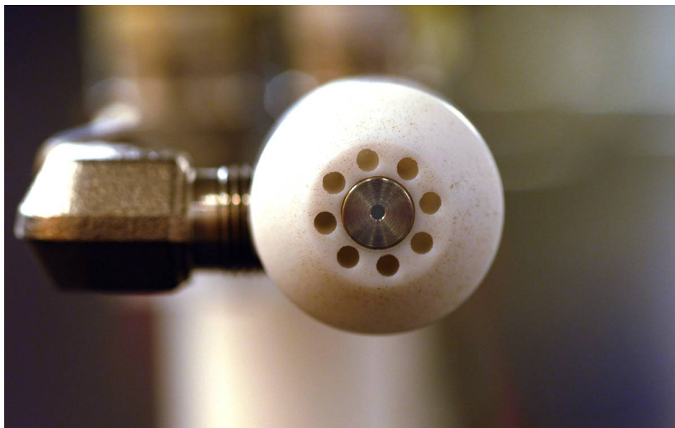
Fig. 2. Detail of the co-axial nozzle. The center hole in stainless steel is the CO 2 snow exit. The multiple holes in the white fluoropolymer are N 2 cover gas exits. (Photograph by Shockey)
