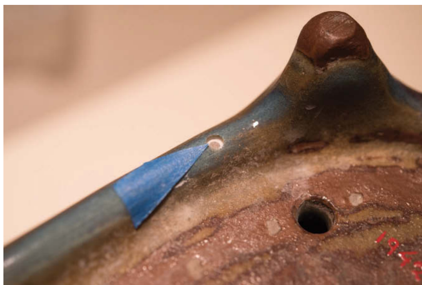
Fig. 12. Resulting 3-mm OD sample hole (Courtesy of Anthony Sigel)
