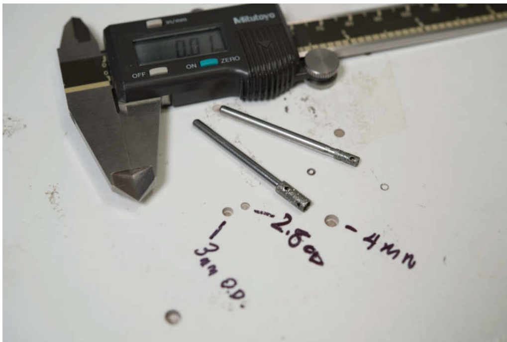
Fig. 2. Digital calipers with diamond core drill sizes, 2.8-, 3-, and 4-mm OD—the most commonly used—and the resulting holes in a ceramic tile (Courtesy of Anthony Sigel)
