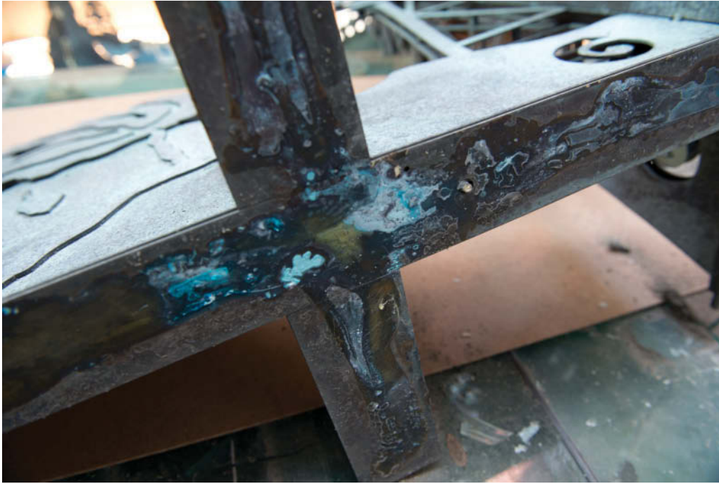
Fig. 8. Detail of suspected bronze disease on the underside of the brass figure, Totem urbain/Histoire en dentelles , 2015 (Courtesy of Alexander Gabov, CSMO)
