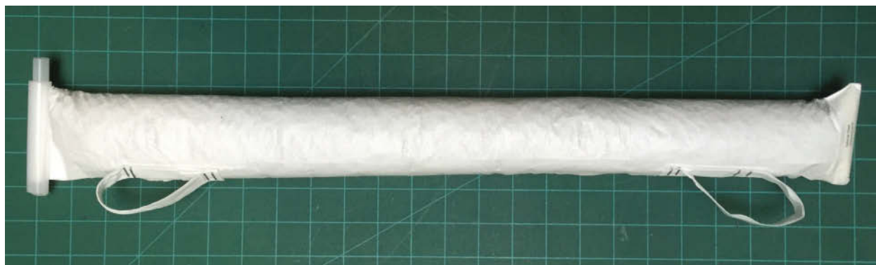
Fig. 4. Completed desiccant tube filled with approximately 900 g activated silica gel (Courtesy of the author)
