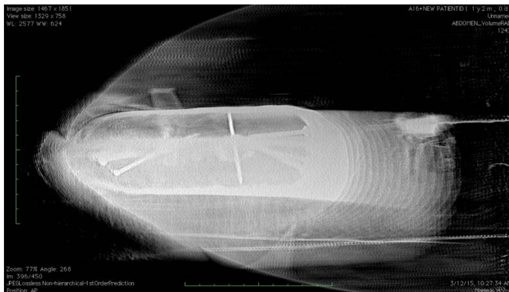
Fig. 9. Projection 13/24 of the axial VolumeRAD sweep of the neck shelf on the Barnes Swan. A pink rectangle indicates the area showing the metal pin securing a metal dowel (Courtesy of Shelburne Museum and UVMCH)
