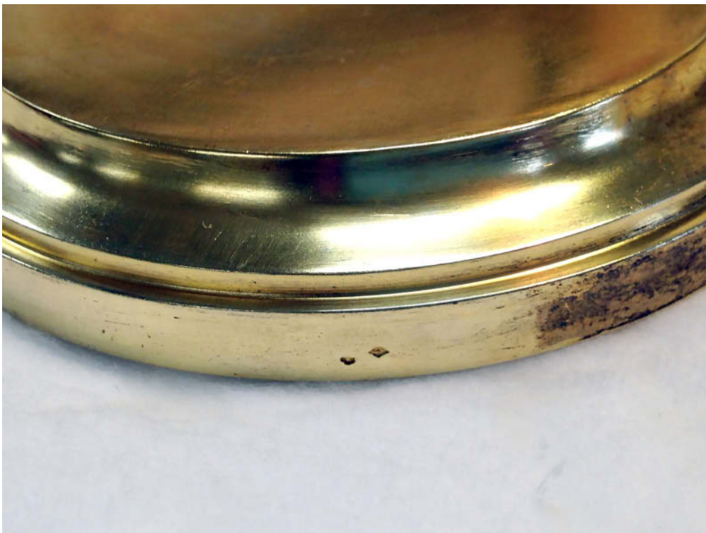
Fig. 12. During tarnish removal of the gilt-silver base, showing two small maker's marks (Courtesy of the author)
