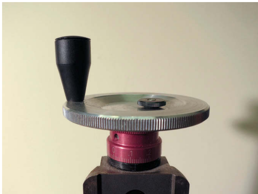
Fig. 7. Handwheel showing graduations and locking knob (Courtesy of Anthony Sigel)
