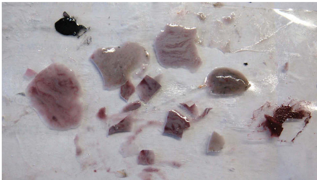
Fig. 12. Creating striated epoxy chips (Courtesy of Historic New England)
