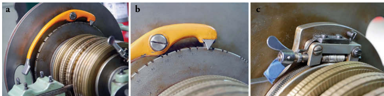
Fig. 18a. Crossing plate and detent; 18b. Crossing plate and detent; 18c. A worm and worm wheel (Courtesy of Brittany N. Cox)
