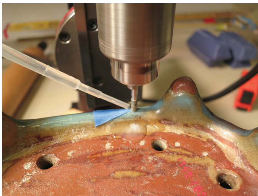
Fig. 8. Keep the bit lubricated with water (Courtesy of Elizabeth La Duc)
