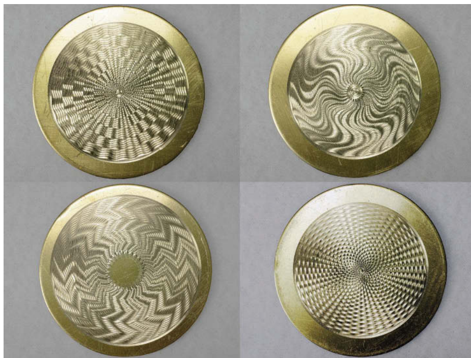
Fig. 19. Four distinct patterns cut with the same rosette and rubber on the rose engine (Courtesy of Brittany N. Cox)
