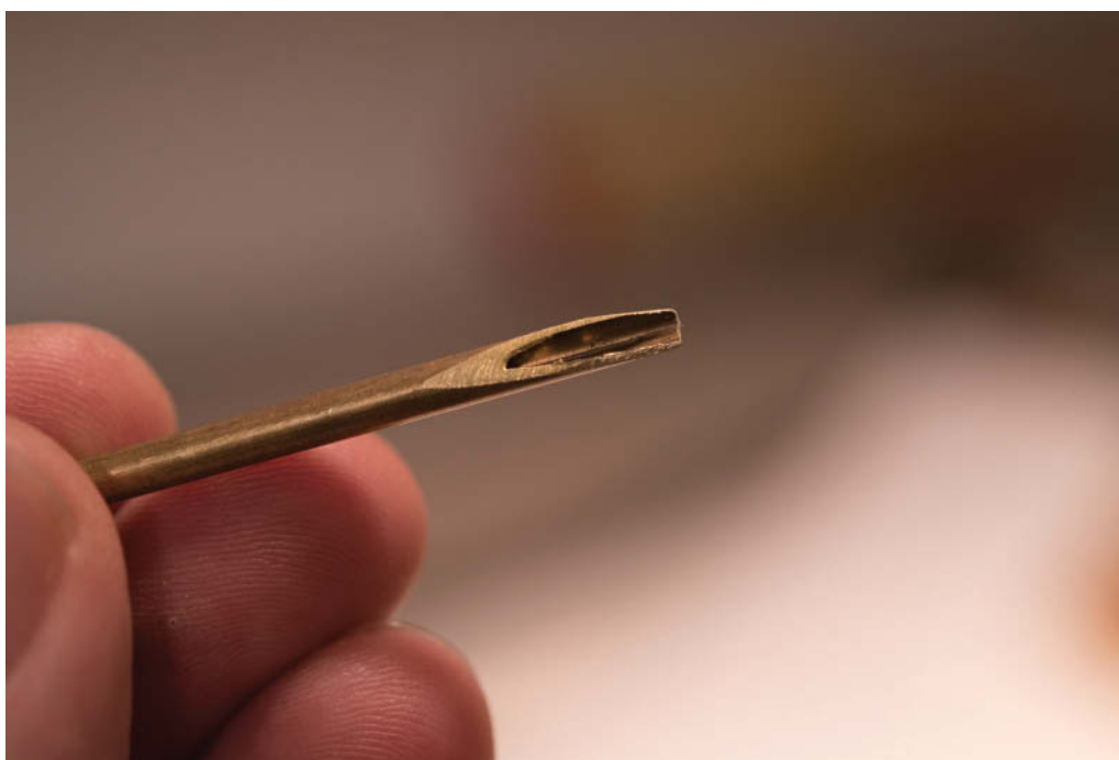
Fig. 3. Brass sample removal tool (Courtesy of Anthony Sigel)
