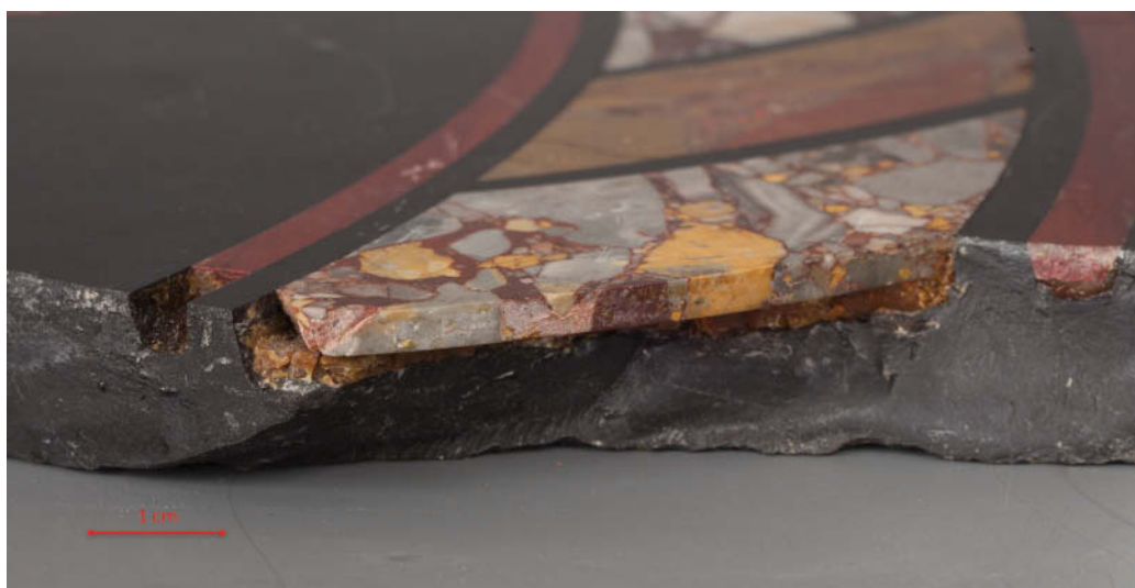
Fig. 2. Break edge of the tabletop illustrating the manufacturing technique of pietre dure . From bottom to top: the black marble substrate, the rosin layer, and the decorative stone slab. Note the thickness of the adhesive layer (Courtesy of Historic New England)
