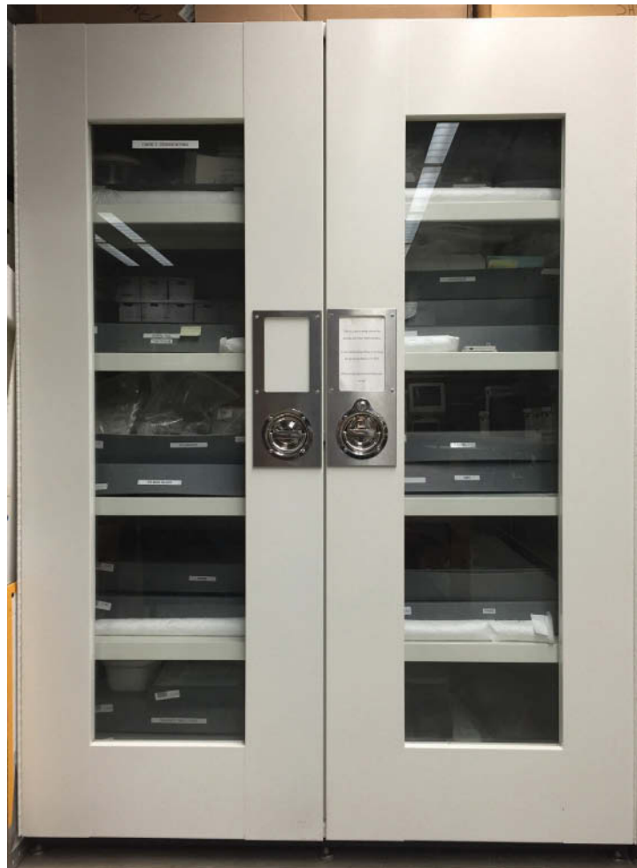
Fig. 2. The Delta Designs DDLX-G cabinet in which the desiccant tubes are installed (Courtesy of the author)
