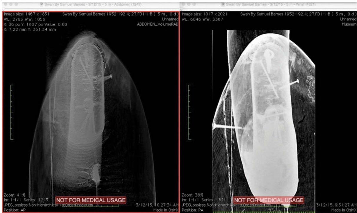
Fig. 8. Projection 7/24 of the axial VolumeRAD sweep of the neck shelf on the Barnes Swan (left) and the posterior-anterior view two-dimensional radiograph of the same area. Pink rectangles indicate the location of the maker's mark on each image (Courtesy of Shelburne Museum and UVMCH)
