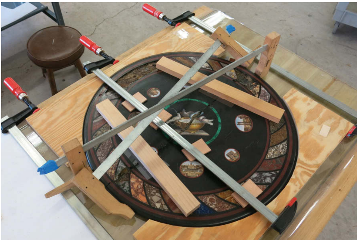
Fig. 8. Clamping system used to join the tabletop sections (Courtesy of Historic New England)
