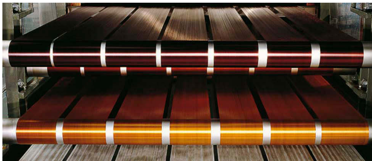
Fig. 1. Polyacrylonitrile (PAN) fibers going through the oxidation process; as PAN fibers oxidize, they change from white to copper, then finally to black (Courtesy of StellaViegas.com.br)
