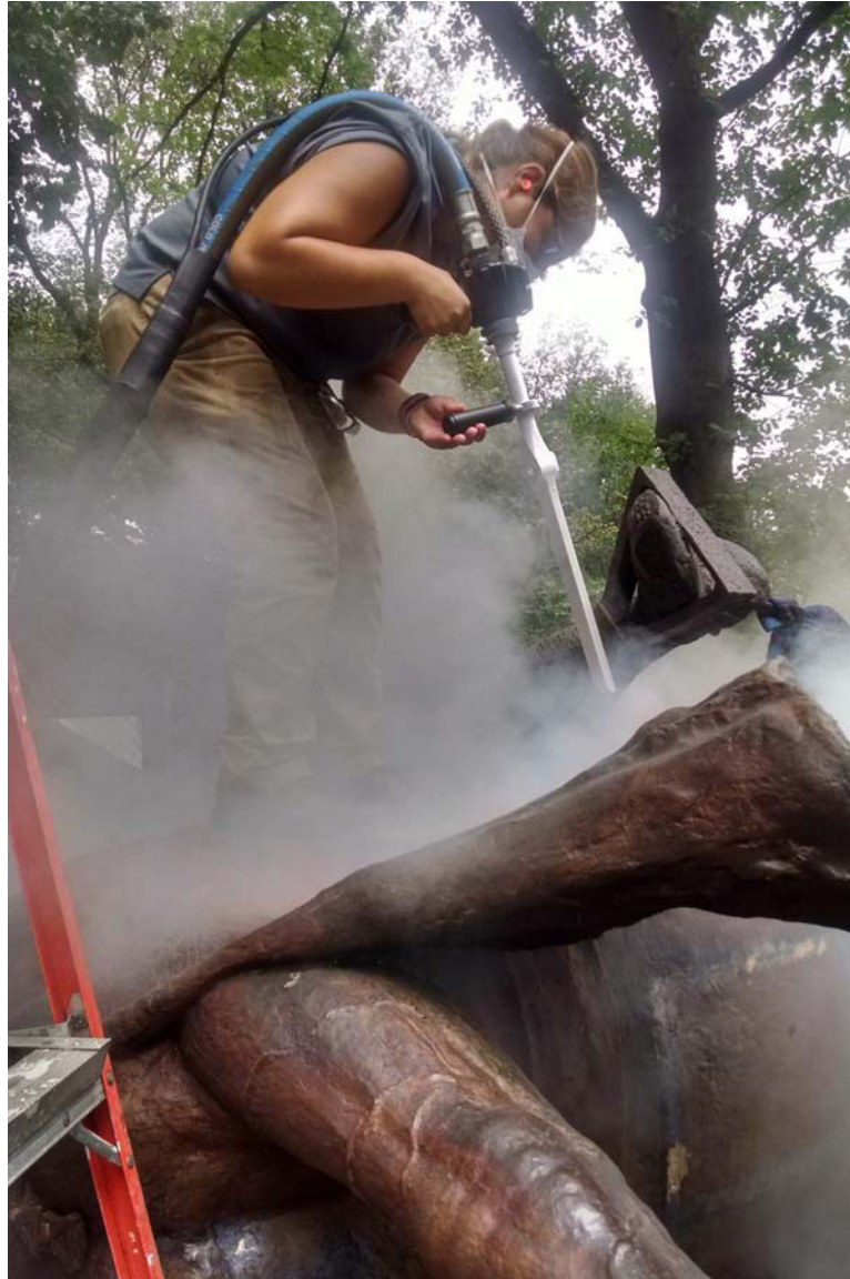
Fig. 10. Dry ice blasting while sculpture was deposited from base
