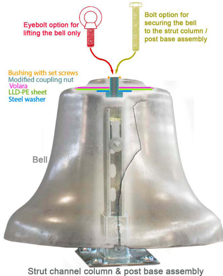
Fig. 7. A diagram illustrating the modified coupling nut, washers, and isolating layers attached to the USS Rainier bell prior to lifting and mounting (US Navy photo by Naval History and Heritage Command Collection Management Facility staff/Released 180305-N-NO147-007)
