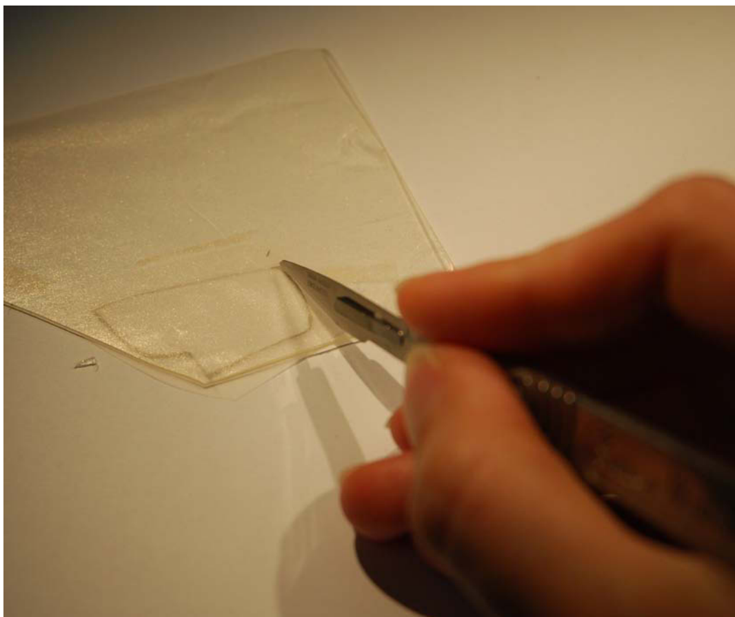
Fig. 7. Cutting the gap fill to size
