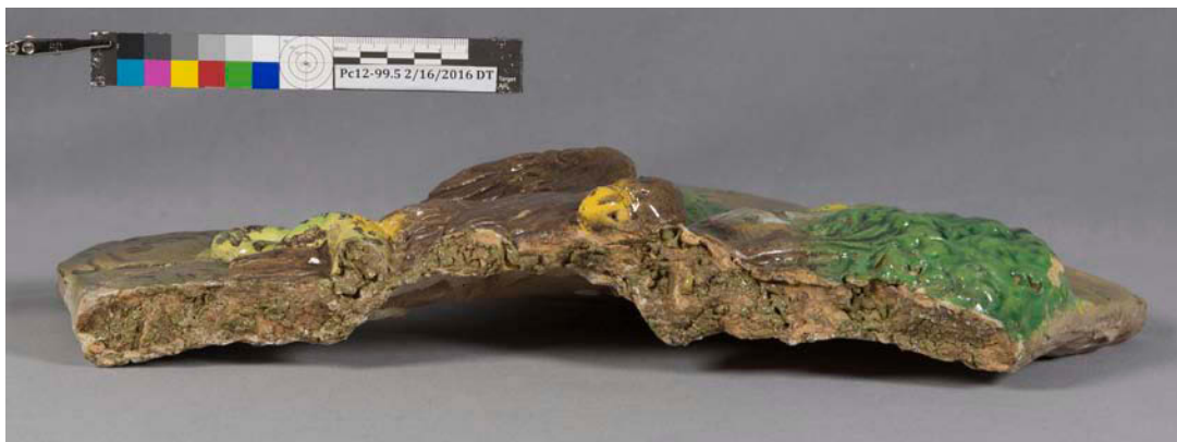
Fig. 13. The break edge of a tile that had been readhered before the second firing with green glaze (Courtesy of the Brooklyn Museum)
