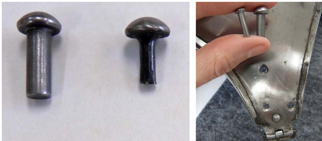
Fig. 12. Comparison of modern commercial rivet (left) and historic restoration rivet (center); commercial rivets held near holes in a breastplate (right).
