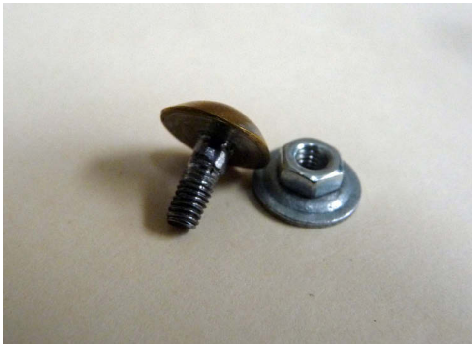
Fig. 7. Assembled, brass-plated threaded fastener with locknut and integral washer, fabricated by armor conservator Ian Ashdown.
