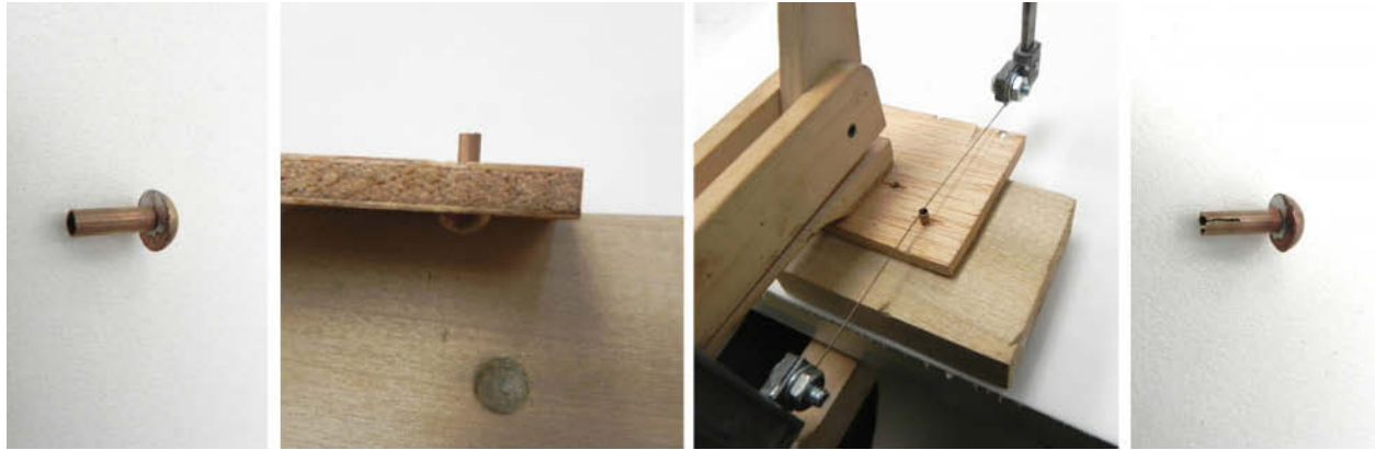
Fig. 10. Steps in fabrication of a split-tube fastener (Courtesy of Philadelphia Museum of Art)
