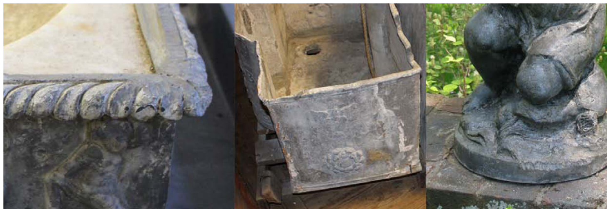
Fig. 4. Details of squirrel damage to lead sculptures
