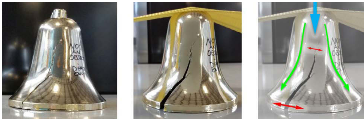
Fig. 5. A mock-up demonstration of stresses that may occur in a cracked bell with the downward force from strapping at the top of the bell or above the waist (US Navy photo by Naval History and Heritage Command Collection Management Facility staff/Released 180305-N-NO147-006)
