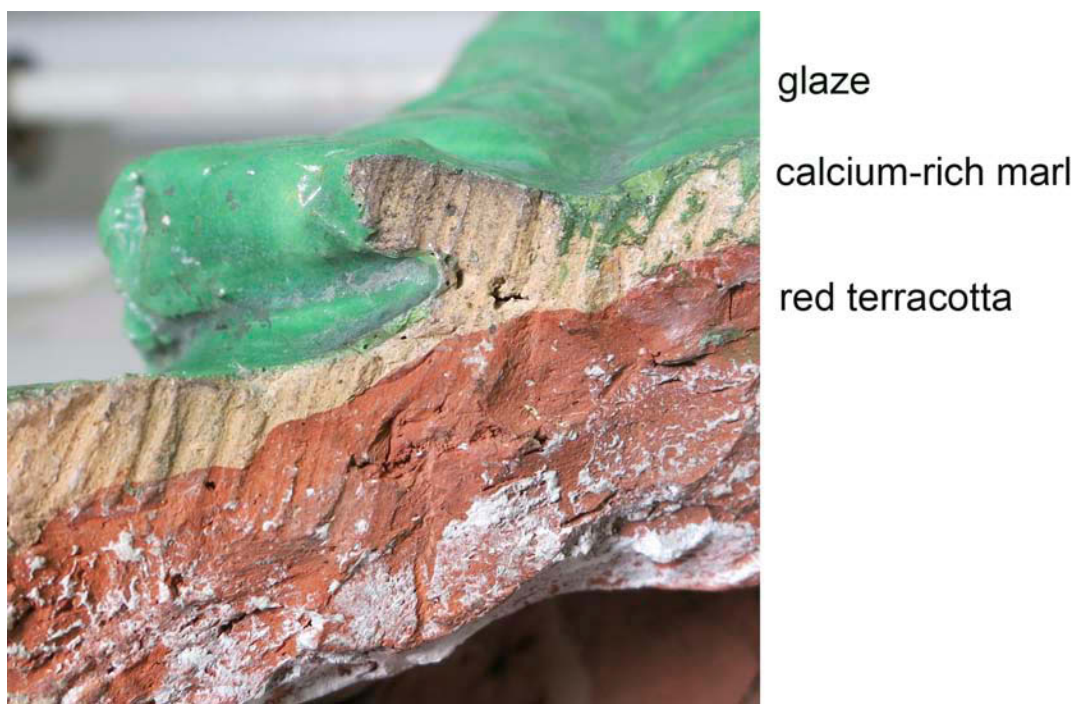
Fig. 7. The side of a border tile, showing the top green glaze layer, thin beige marl, and thick red terracotta substrate. Green restoration paint and plaster residues are also present (Courtesy of the Brooklyn Museum)
