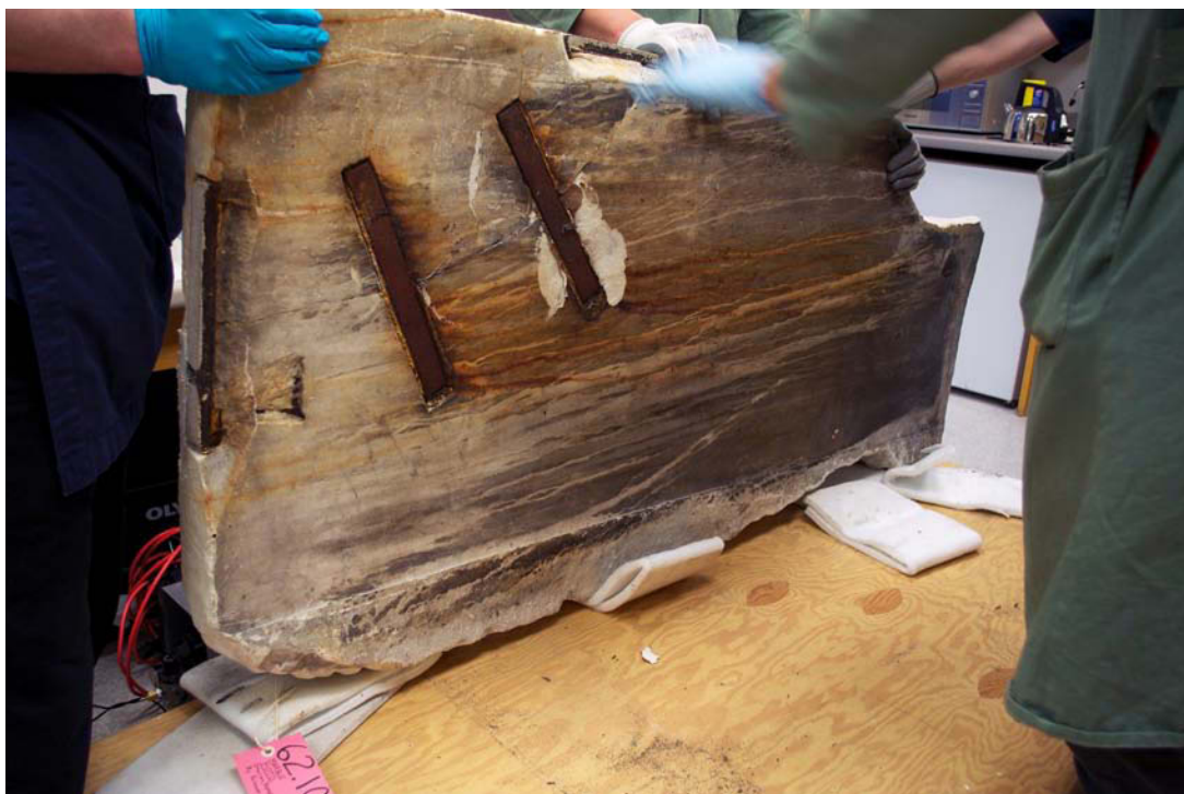
Fig. 5. The cramps and the resultant staining on the verso of the relief fragment (Photograph by Rachel C. Sabino, courtesy of the Art Institute of Chicago)
