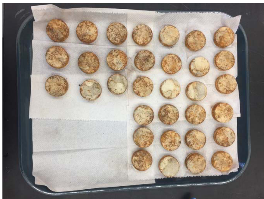
Fig. 4. Marble samples after staining
