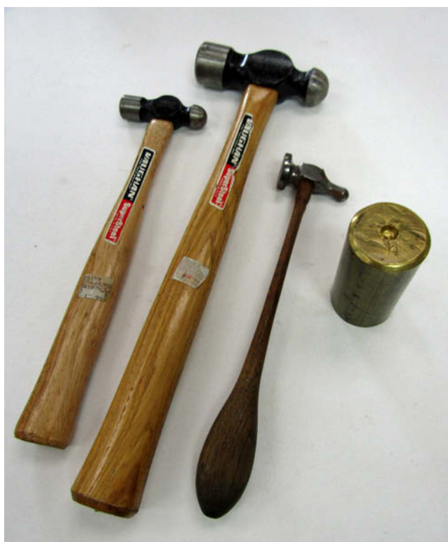
Fig. 13. Rivet set and ball peen hammers (Courtesy of Philadelphia Museum of Art)
