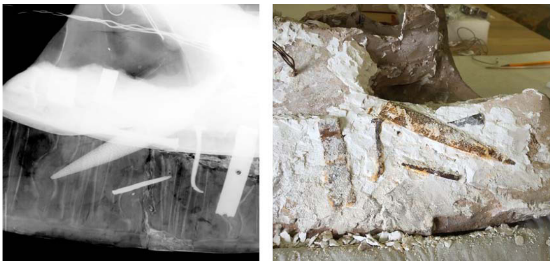
Fig. 6. Left: x-ray radiograph (80 kV, 1.5 mA, 5 s, Cu filter) of Christ's legs, proper right side; Right: the same area shown during treatment as metal elements embedded in plaster were exposed (Courtesy of the Brooklyn Museum)
