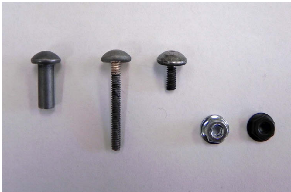
Fig. 8. Fabrication of a threaded fastener at PMA: reused or new rivet head soldered to a threaded rod, and locknut with an attached washer darkened for use on the interior (Courtesy of Philadelphia Museum of Art)
