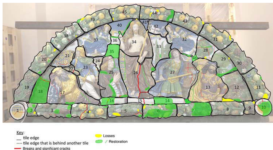
Fig. 3. Condition diagram before the tiles were removed from the backboard (Courtesy of the Brooklyn Museum)
