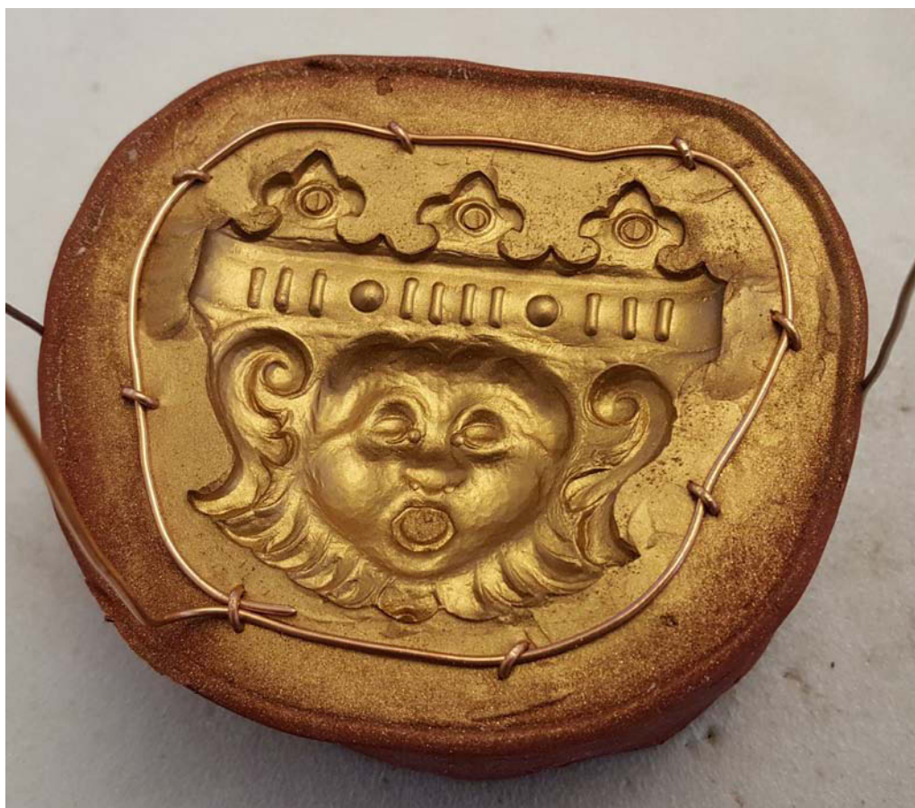
Fig. 3. Silicone rubber mold prepared with copper perimeter wire and dusted with bronze powder
