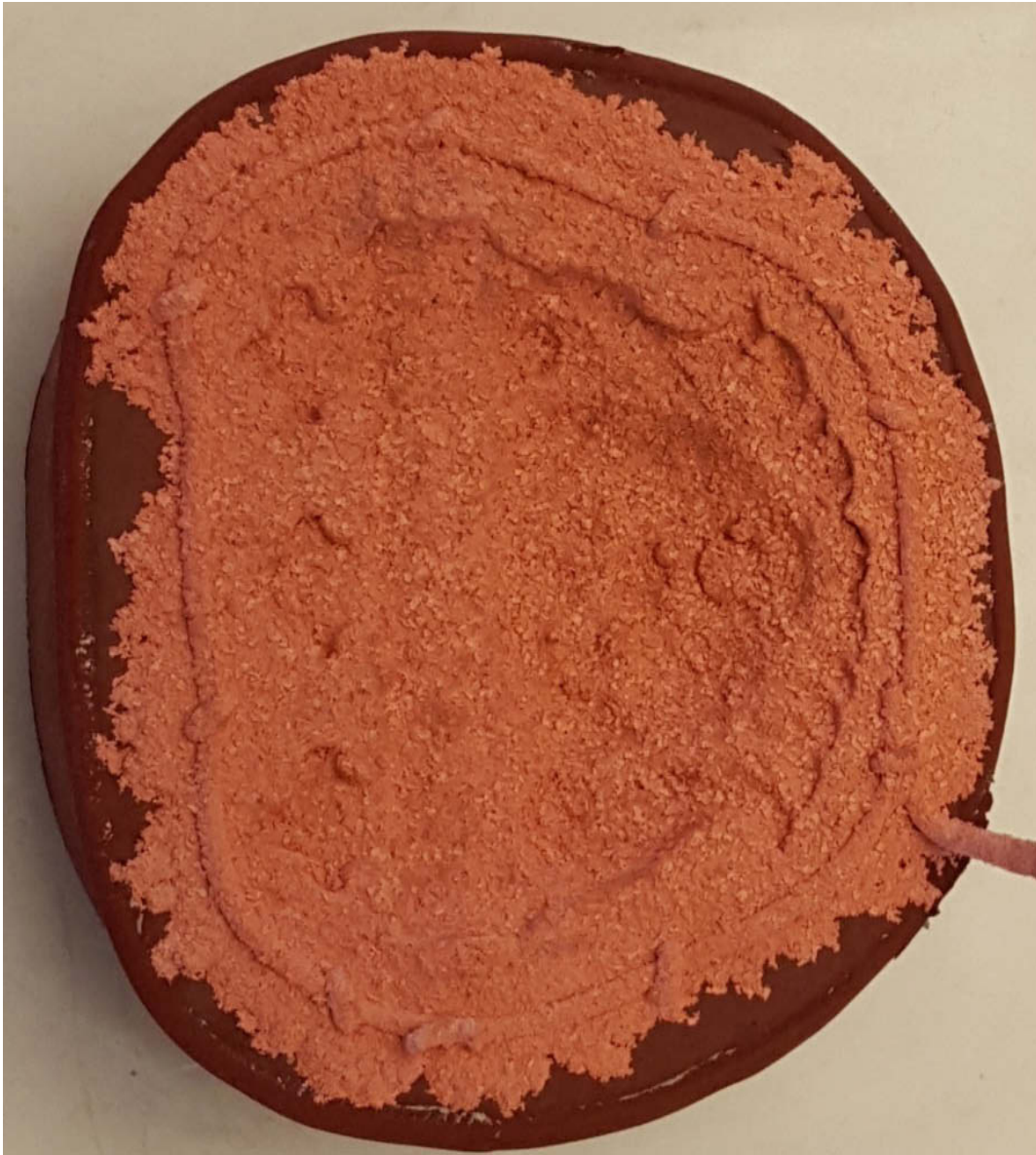
Fig. 5. Freshly electroformed copper, illustrating its coarse crystalline growth habit
