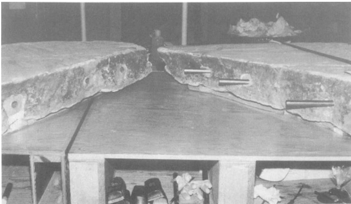
Figure 13. Top break edge with parallel dowels in place.
