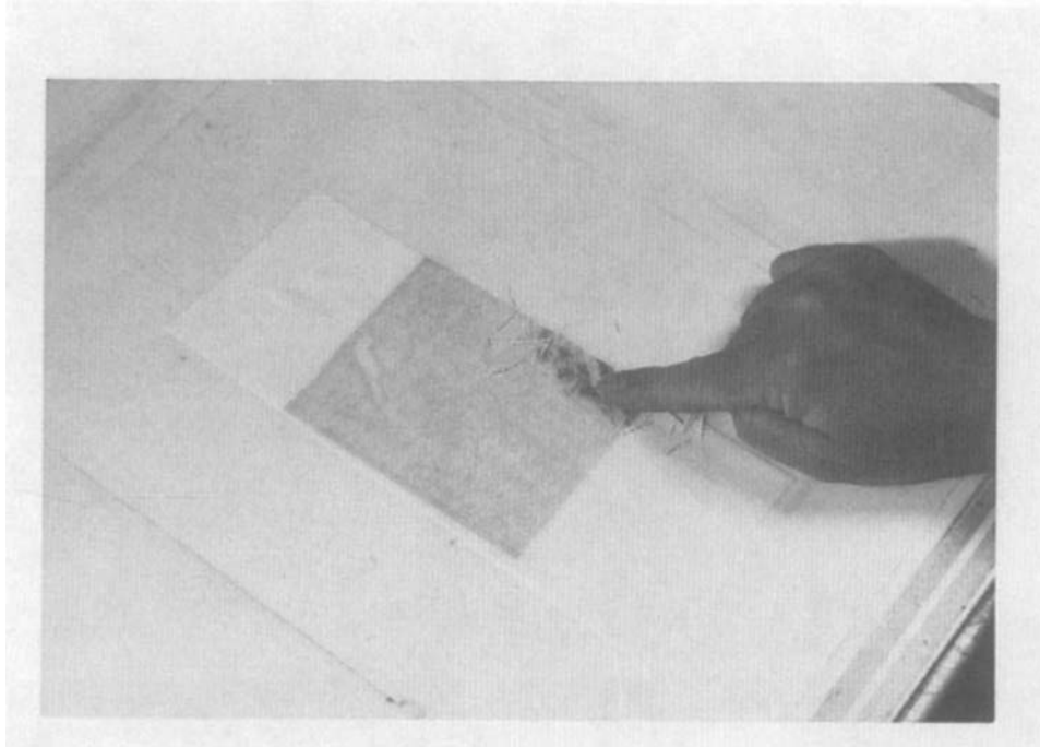
Figure 6: The swelled and softened paper is removed from the image.
