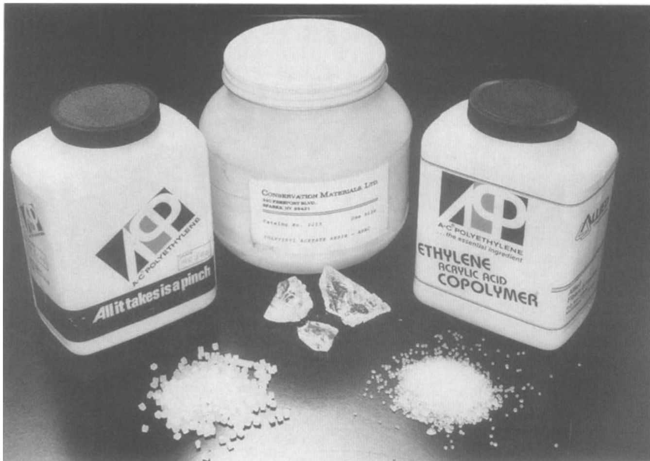
Figure 1. The different components that constitute the wax-resin fill material.
