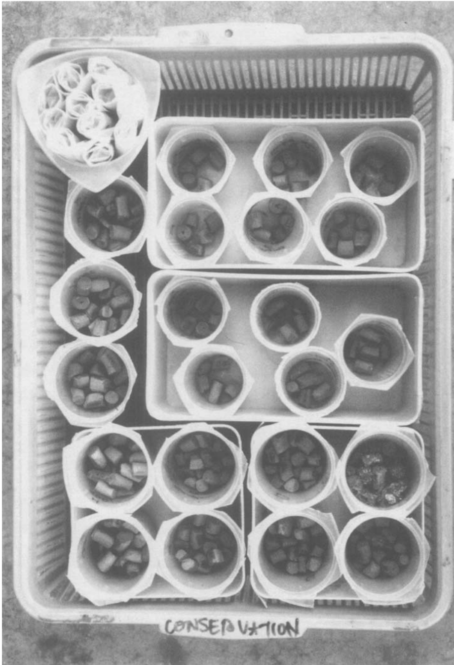
Figure 4. Real-time aging experiment (February 1999). Samples are stored in large cups by desalination group (small cups are subsets of these), with some in closed polyethylene bags (upper right corner). Group A samples (undesalinated control) show white fluffy salt efflorescence (large cup near the lower left corner) and delaminated ceramic surface (small cup in the lower right corner).
