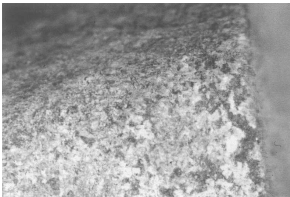
Figure 6. An undersalinated sample stored in a cup, after 4 years (20x magnification). A whitish crust has developed on the exterior surface, containing calcium sulfate dihydrate (gypsum) with some sodium chloride, as analyzed by XRD.
