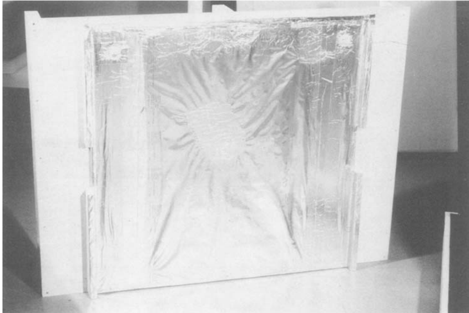
Figure 21. Installation Tray. 46" x 36". Plywood with footprint of the object. The rim around the footprint and the footprint are covered with Marvel-seal, which is heat-sealed. The footprint of the object aligns with the edge of the installation crate (edge seen at the floor).
