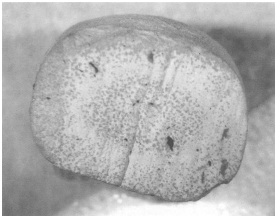
Figure 7. A sample desalinated to 400\mu\text{S}/\text{cm} , after 4 years (8x magnification). The cut surface exhibits fine reddish brown spots in the center and concentrated near outer edges.
