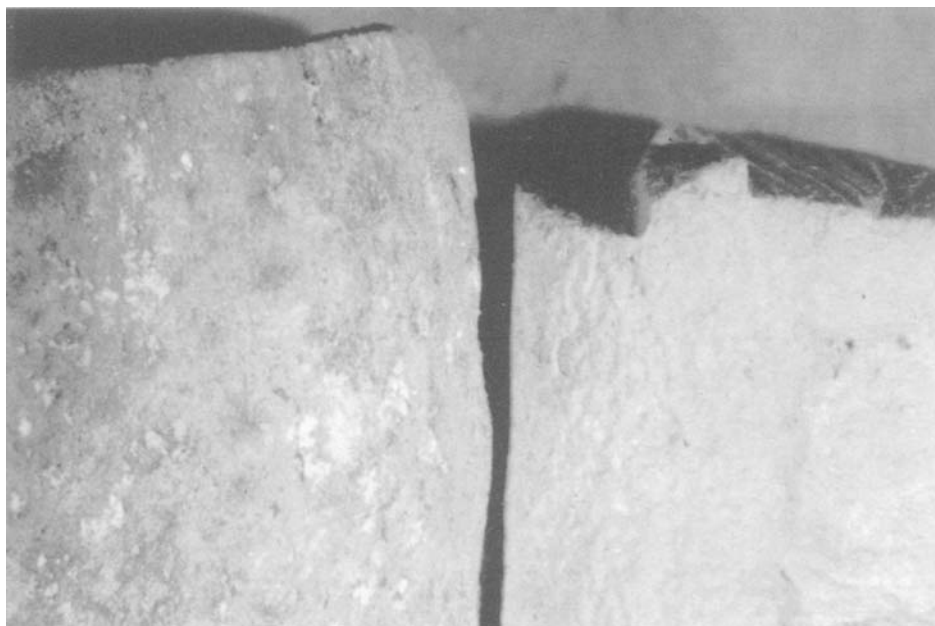
Figure 5. Two samples from the same original bangle fragment, stored in cups (8x magnification). The undersalinated control (left) shows white fluffy salts, while no changes are visible on the sample desalinated to 400\mu\text{S}/\text{cm} (right), after 4 years.
