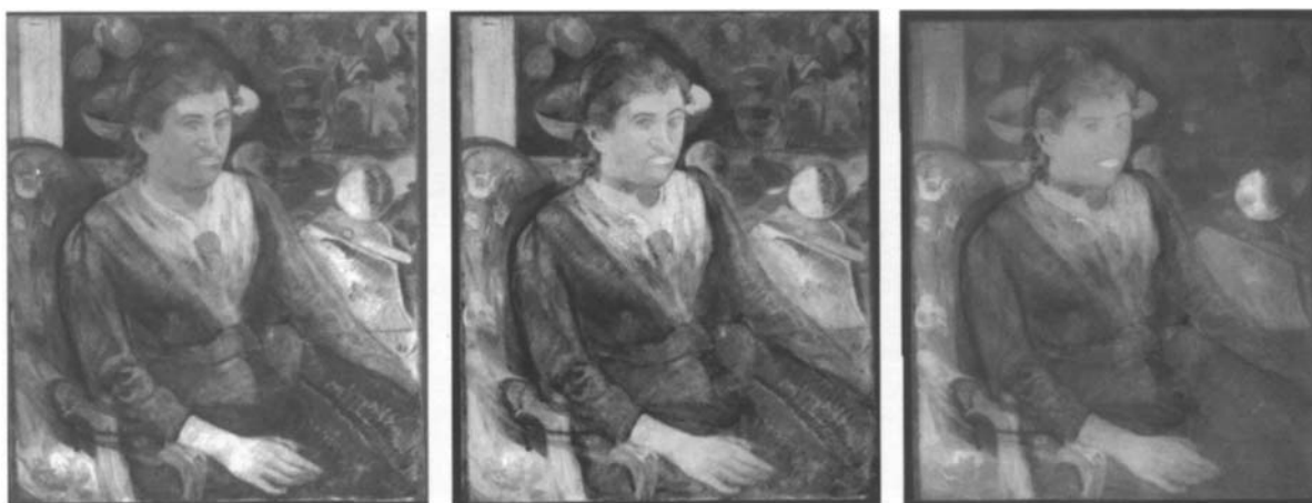
Figure 15 Paul Gauguin Portrait of a Woman with Still Life by Cézanne three overall reflectograms taken with 1.1-1.4 micron filter, 1.5-1.8 micron filter, and 1.9-2.4 micron filter respectively.
