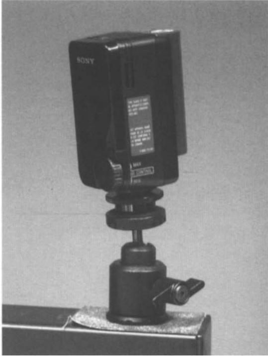
Fig. 9 Detail of Sony battery-powered infrared light source (Model #HVL-IRC).
