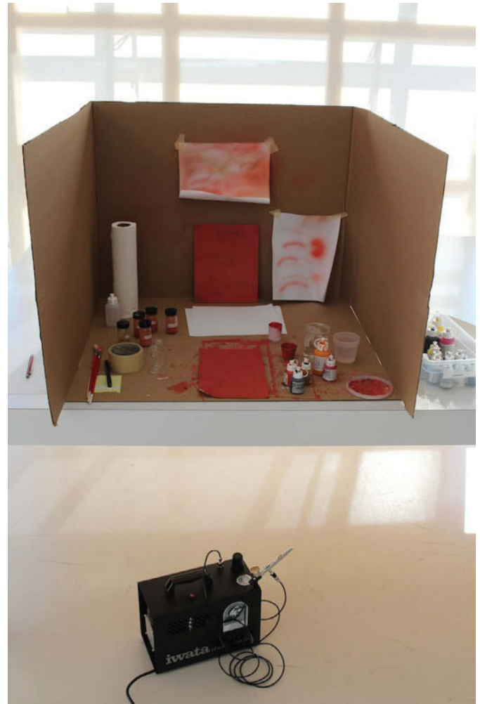
Figure 3. Mini-spray booth built of cardboard for testing or small-scale projects
