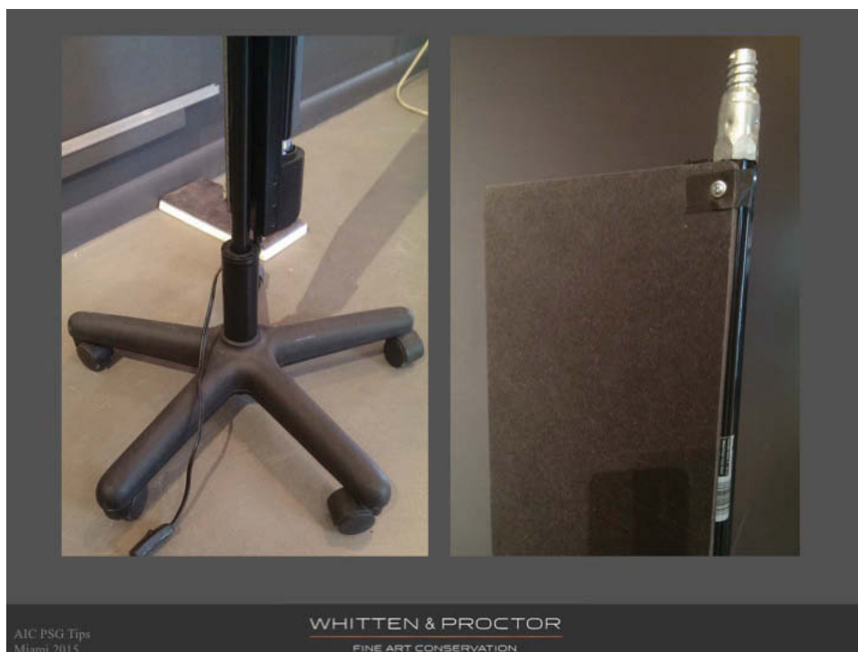
Figure 1. Salvage wheels and base from office chair for light stand
