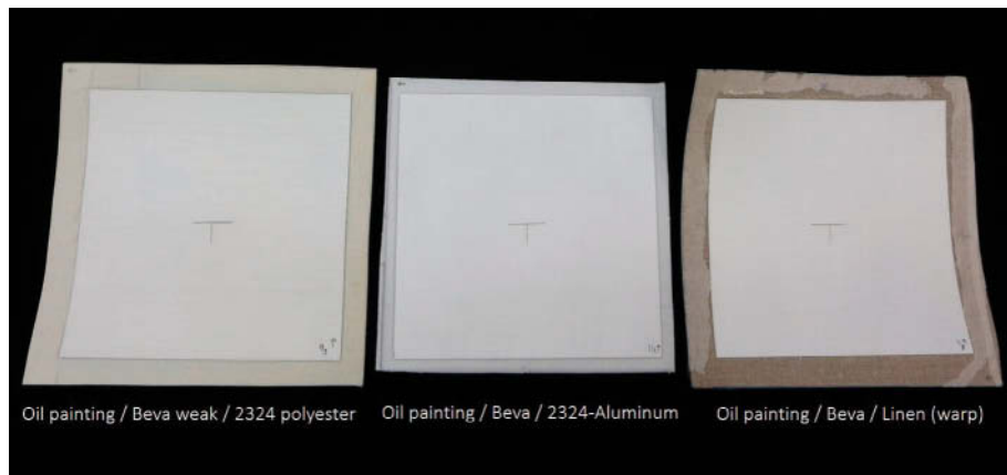
Figure 12. Biaxial samples prepared with a “tear-cut” in the center of the model painting prior to lining. The center sample is marouflaged onto aluminum; the other lined samples were left free floating. © Government of Canada, Canadian Conservation Institute, CCI 86055-0343
