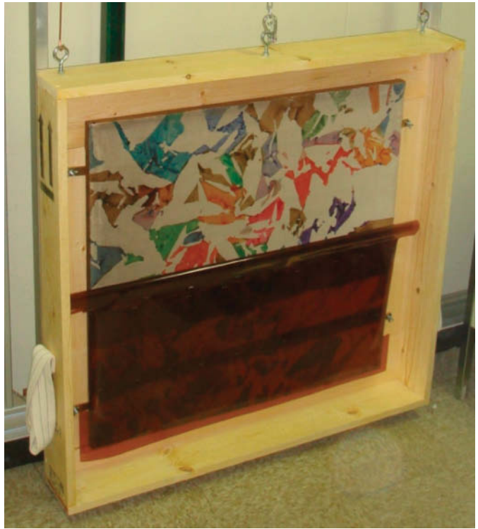
Figure 10. The painting masked with polyimide film in preparation for atomic oxygen cleaning tests; Simon Hantaï, 1973, acrylic and exposed ground on canvas, 29 3/4 × 30 1/4 in. Courtesy of NASA
