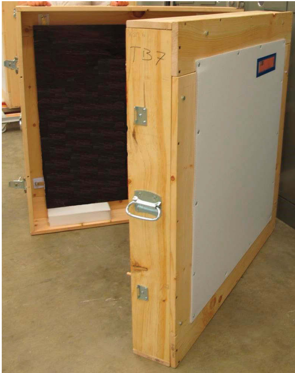
Figure 4. A two-painting travel box. Each painting is secured with Oz Clips attached to each face of the travel box. There is ample gap between the paintings, which ensures that there is no surface contact between them
