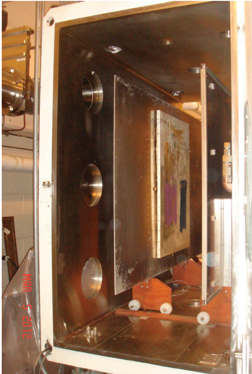
Figure 12. One panel of the multipart painting installed in the atomic oxygen chamber at the Glenn Research Center; Joan Mitchell, 1971, oil on canvas. Courtesy of NASA
