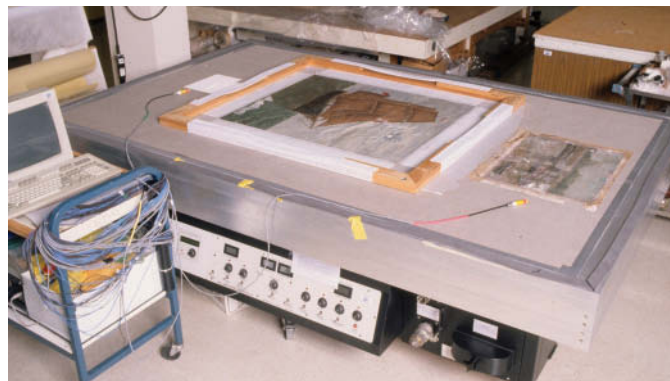
Figure 3. In the early monitoring system, temperature and humidity probes were placed under one or more experimental paintings, placed to the side of the painting being treated. © Government of Canada, Canadian Conservation Institute
