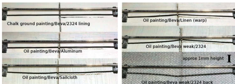
Figure 13. Photographs of “paintings with a tear” on various linings, after 18 years at room conditions. A straight pin is illuminated from overhead, its shadow (the solid dark line) reveals the cupping. © Government of Canada, Canadian Conservation Institute, CCI 86055-0315
