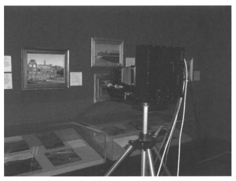
Fig. 2. The new SIRIS infrared camera in use at the National Gallery, London to image a painting  $in \, situ$
