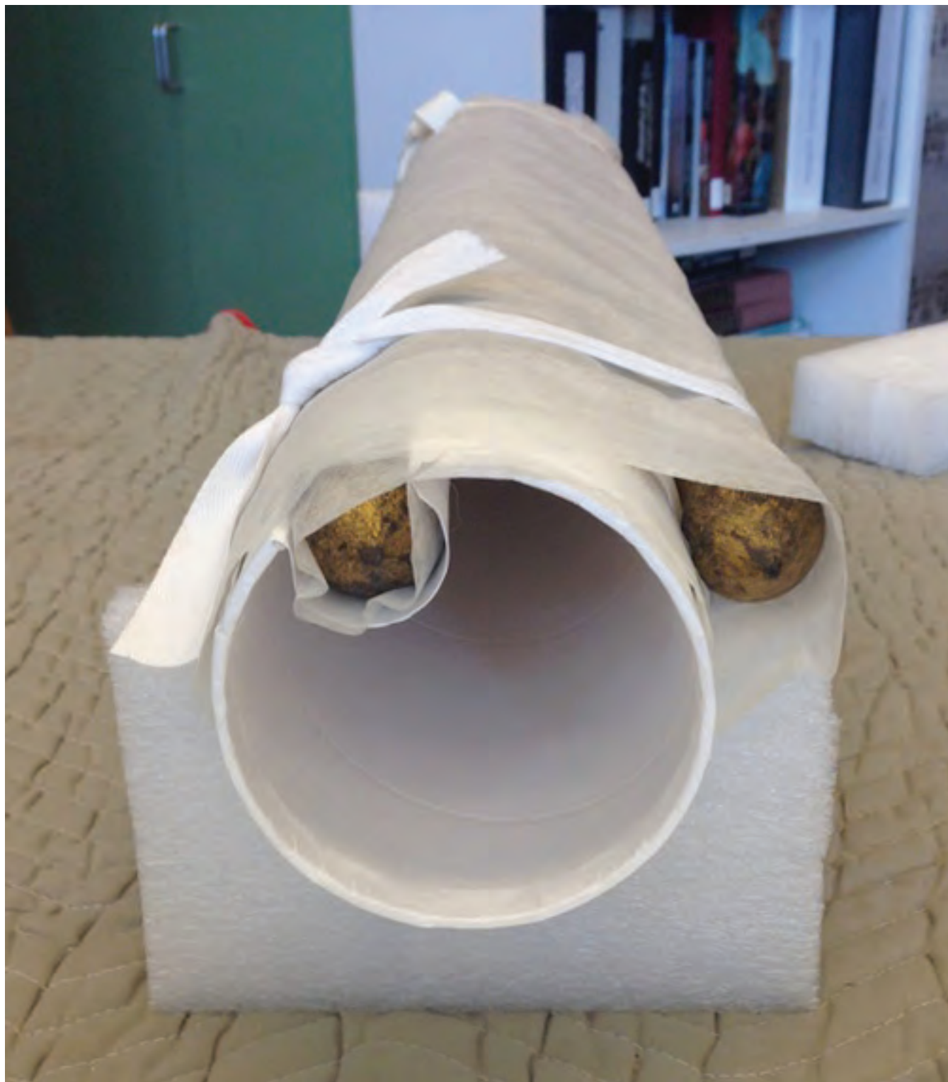
Figure 20. Detail of painting rolled on modified roller resting on foam cradles.
