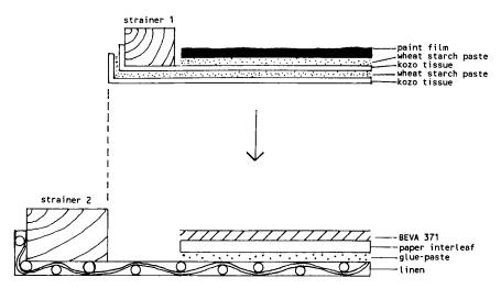
Figure 2: The lining setup and the structure of the support (not to scale).
