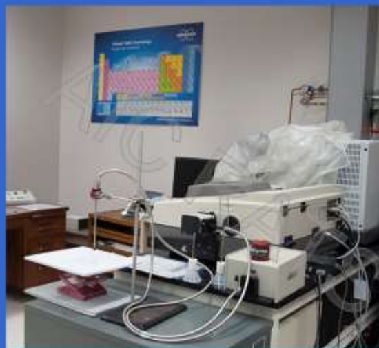
Fiber-optic reflectance probe and detector (Remspec Corporation) attached to FTIR spectrometer
