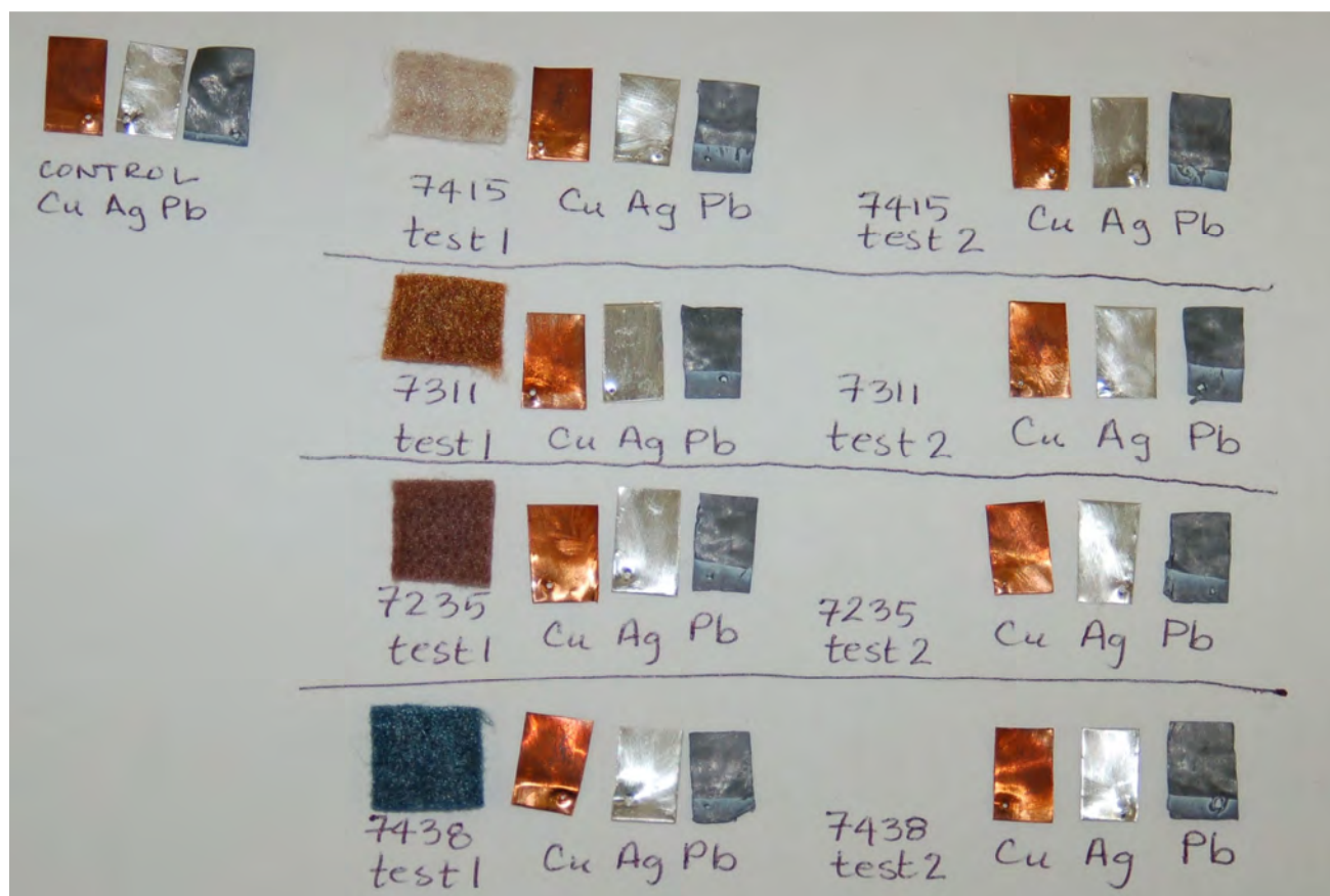
Figure A1: The appearance of the metal coupons after 28 days of heating; the coupons on the left were contained in the control tube and those on the right were contained with each felt sample.
