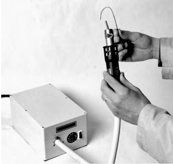
FIG. 5 Bending the material with a Leister hot air tool.
