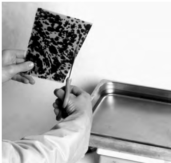
FIG. 4 Warming the material in hot water and cutting with scissors.
