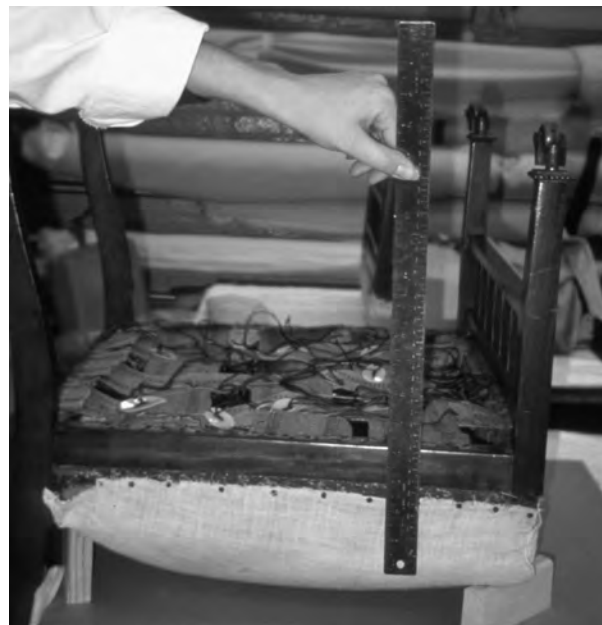
FIG. 2 Measuring to determine appropriate height of springs. Note support used to elevate seats to avoid over-compression or flattening of seat profile. Courtesy New York State Office of Parks, Recreation and Historic Preservation, Olana State Historic Site.
