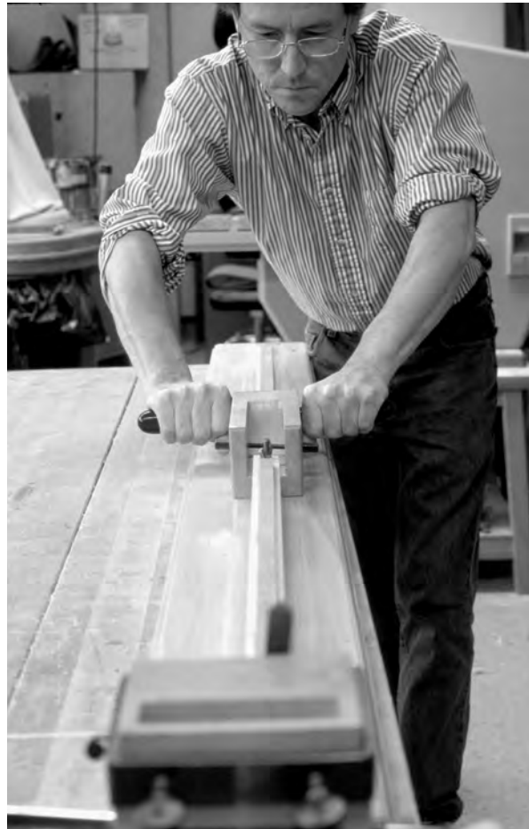
FIG. 8 Making a molding on the Moxon “Waving Engine.”
