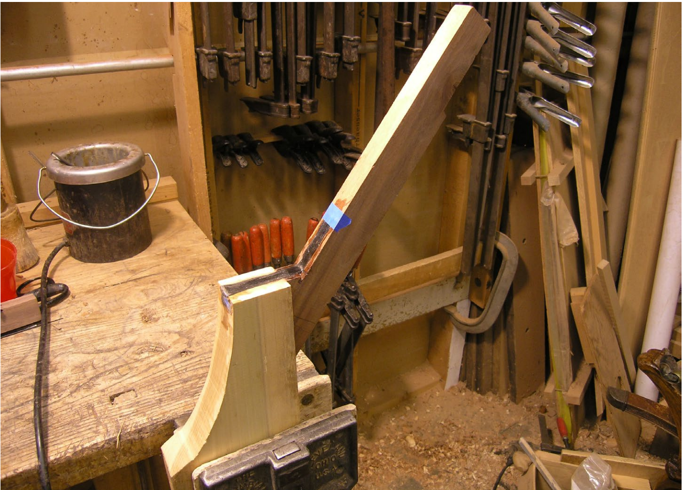
Fig. 10. Set up of a trial testing the efficacy of a carbon fiber-reinforced leg/column joint. The carbon fiber is the only attachment between the 'leg' and 'column'. Nevertheless it held 145 pounds hanging from the end of the 'leg'.
