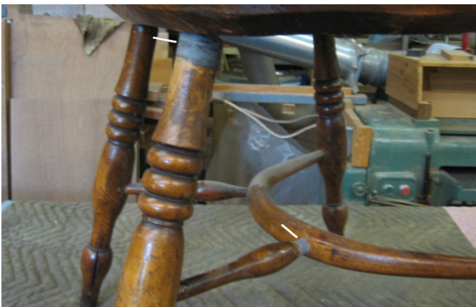
Fig. 21. Bands of carbon fiber-reinforced epoxy on the leg and stretcher.
