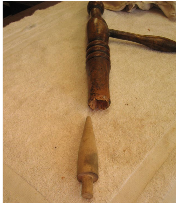
Fig. 17. Turned plug to fit into the leg end and the chair seat.
