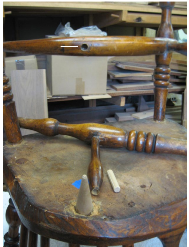
Fig. 18. The plug inserted into the bottom of the chair seat and a dowel ready to be inserted into the end of the broken stretcher.
