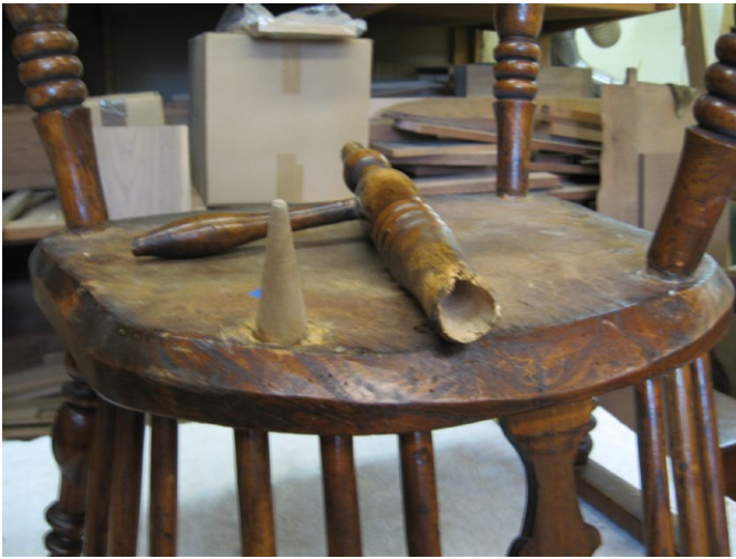
Fig. 19. Another view of the prepared leg and plug.
