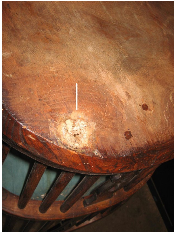
Fig. 15. Underside of a Windsor chair where the insect damaged leg snapped off.
