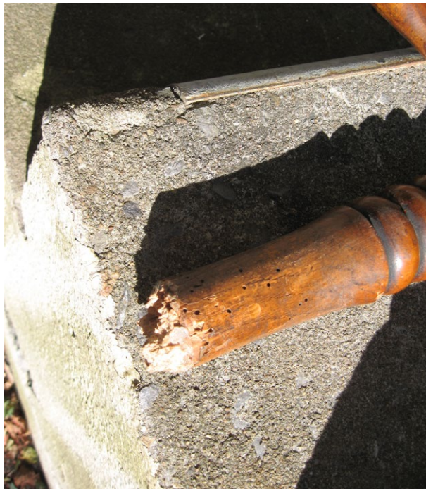
Fig. 16. The end of the leg of fig. 15, showing insect exit holes.
