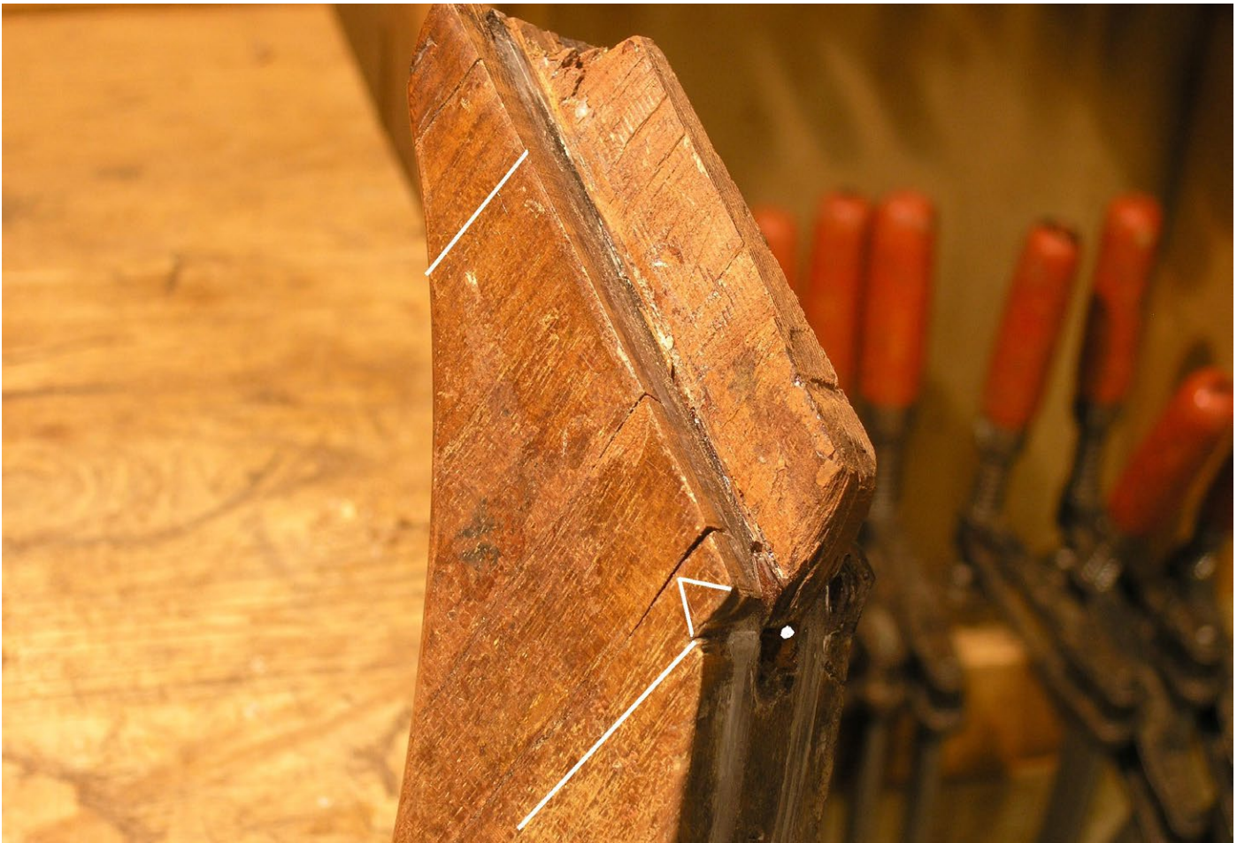
Fig. 4. Pedestal leg showing grain direction in upper leg (indicated by white lines) and resulting split (arrow). This layout is the opposite of the bottom leg in fig.1. Very possibly the maker wanted to give maximum strength to the foot end of the leg, thinking that the column would help strengthen the short grain in the upper part. Not a bad thought, but in this case it didn't work.
