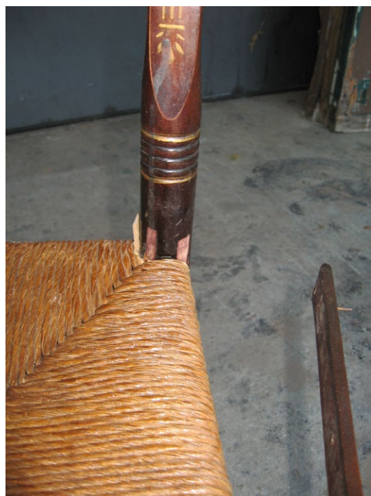
Fig. 25. The finish scraped off the front of the leg in preparation for gluing on carbon fiber reinforcing strips.
