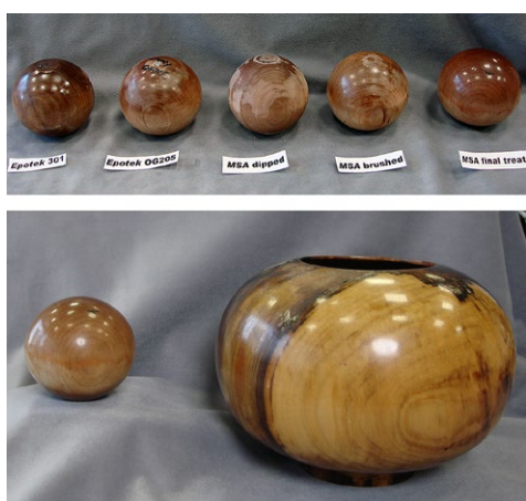
Fig. 4. (a) Visual appearance of 3D PEG 1500-impregnated birch balls with epoxy and Golden MSA-based coatings (b) Visual comparison of mock-up versus original coating on a privately owned bowl Moulthrop tulipwood bowl
