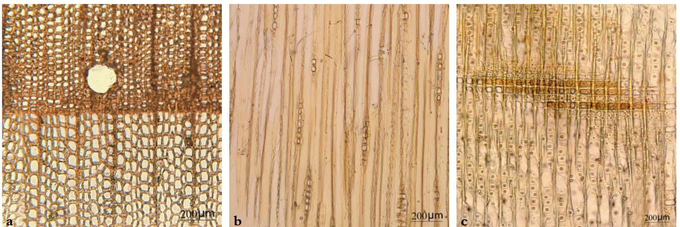
Fig. 2. (a) Transverse section. (b) Tangential section. (c) Radial section.
