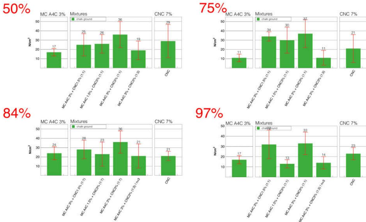
Fig. 5. Tensile strength results after 3 months.
