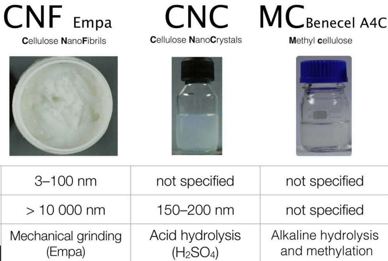
Fig. 2. Suspensions of CNF 3 wt%, CNC 3 wt%, and solution of MC A4C 3 wt%, and their characteristics and production.
