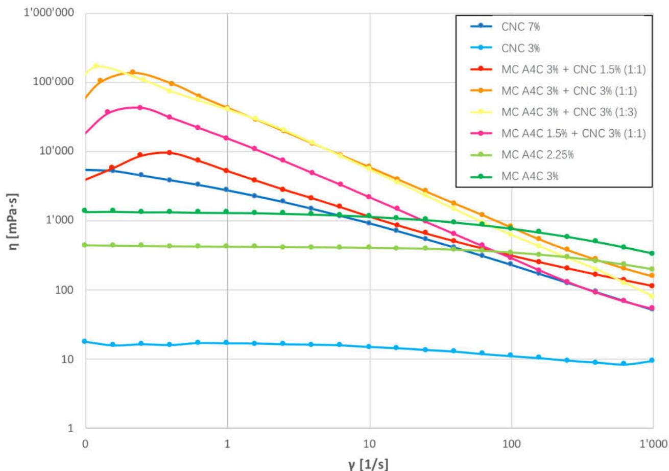
Fig. 3. Viscosity of the suspensions, mixtures, and MC solutions.
