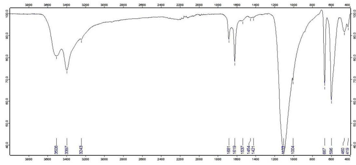
Fig. 4. FTIR results of the ground layer.
