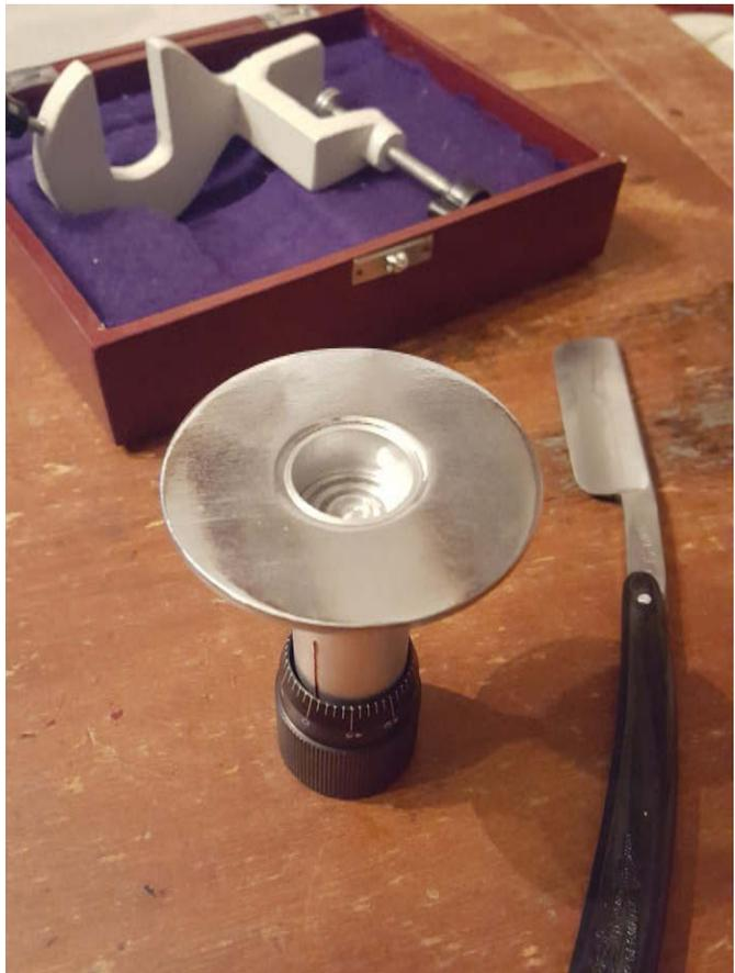
Fig. 2. Example of a commercially available hand microtome.
