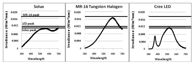
Diagram 2: Spectral power distributions of three lamps – Solux 4700°K, Tungsten Halogen, and a 3500°K LED. All lamps normalized to 660 Lux to match scale in Diagram 1. Horizontal lines placed at  $0.0165W \cdot m^{-2} \cdot nm^{-1}$  for the MR-16 peak,  $0.012W \cdot m^{-2} \cdot nm^{-1}$  for the LED peak, and  $0.011W \cdot m^{-2} \cdot nm^{-1}$  for the Solux peak.
