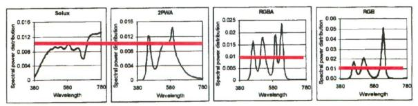
Diagram 1: Spectral power distributions (SPD) of four lamps - Solux and three types of LEDs. These are the graphs accompanying the *Extreme Caution* posting: "Each of the SPD's has a heavy horizontal line at  $0.01W \cdot m^{-2} \cdot nm^{-1}$ , the highest power output of a broad, continuous incandescent lamp".
