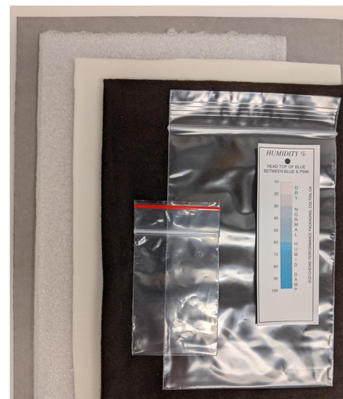
Use inert materials such as (left to right): acid free board, polyethylene foam sheet, Volara, Pacific Brand Silver Cloth, polyethylene bags, and humidification monitors.
