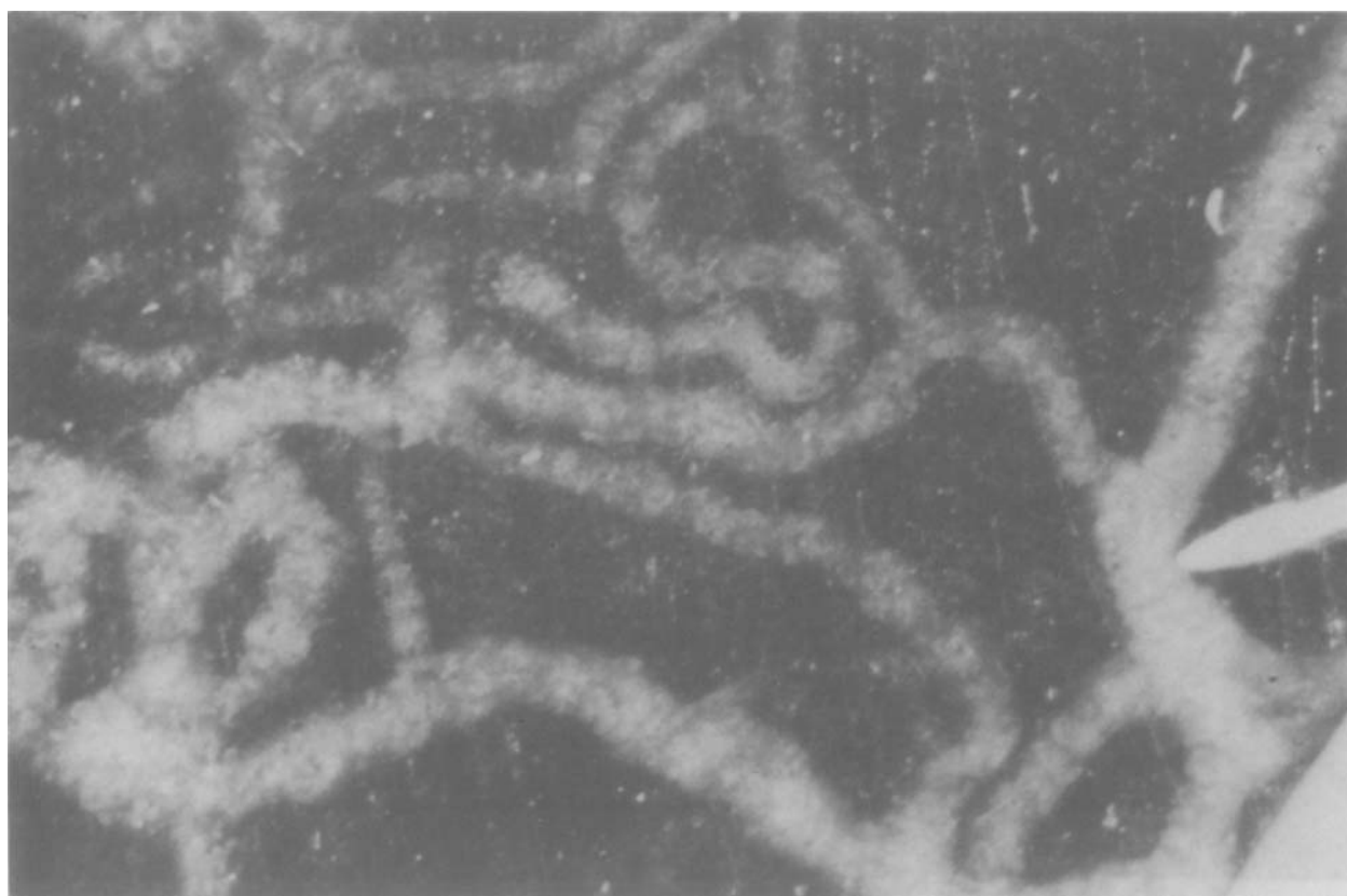
Figure 5. Photomicrograph of filiform corrosion on magnesium support of Cricche Panel 6.
