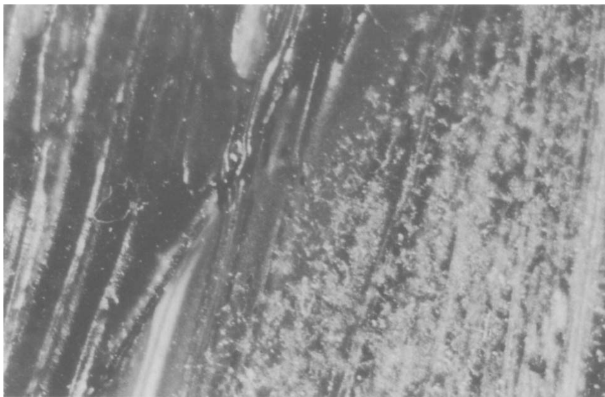
Figure 3. Photomicrograph of masking tape remnants under red paint of Cricche Panel 6. The left portion of the image shows an area where there are no crystals due to the underlying tape.
