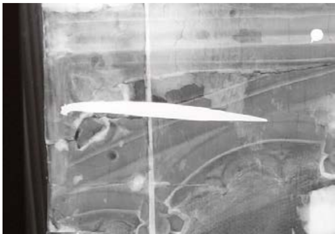
Figure 6. X-radiograph detail of a metal dowel. Jaume Mateu, The Birth of the Virgin , c. 1430–35, tempera and tooled gold on wood panel, 31 1/4 x 22 3/4 x 13/16 in. (79.4 x 57.9 x 2.0 cm). Philadelphia Museum of Art, Johnson Collection, Inv. 2493. © Philadelphia Museum of Art, Conservation Department, Joe Mikuliak.
