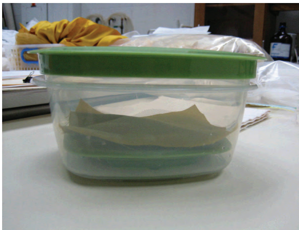
Figure 12. Samples were placed in a humidity chamber buffered to a RH of approximately 70-75%. After prolonged exposure, the adhesive was observed to penetrate and stain the silk habutae.
