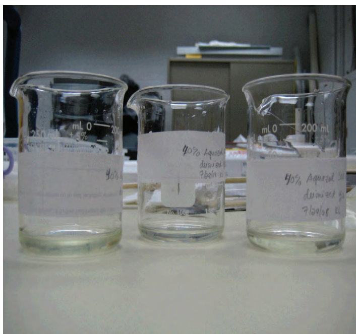
Figure 2. 40% stock solutions of all three molecular weights were prepared using deionized water (on left). Figure 3. Silk crepeline, silk habutae, and Dukeries monofilament nylon net were used as carrier fabrics (on right).
