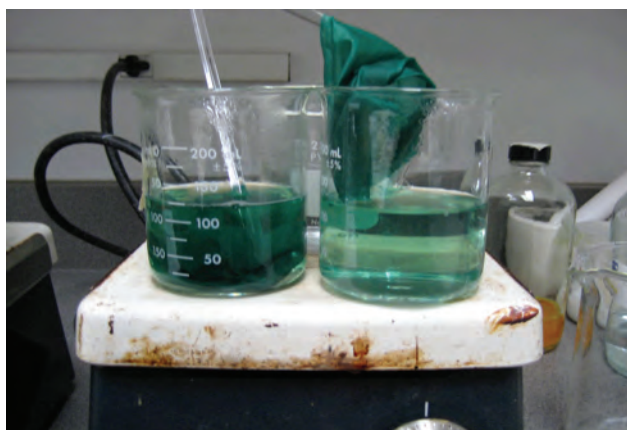
Figure 7. Nylon net and silk habutae were custom dyed to match the original fabric color using Lanaset dyes.
