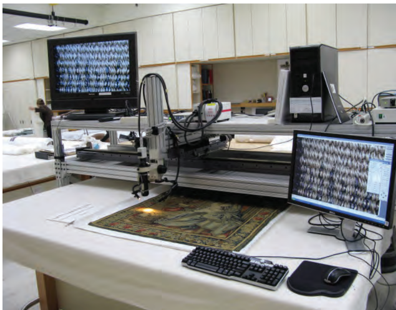
Figure 2. Wide span bridge over worktable. HD camera fitted with Navitar lens on motorized arm. The large flat screen monitor (left) shows the HD analog image and the computer screen (right) shows the processed digital image. Photo 2009.
