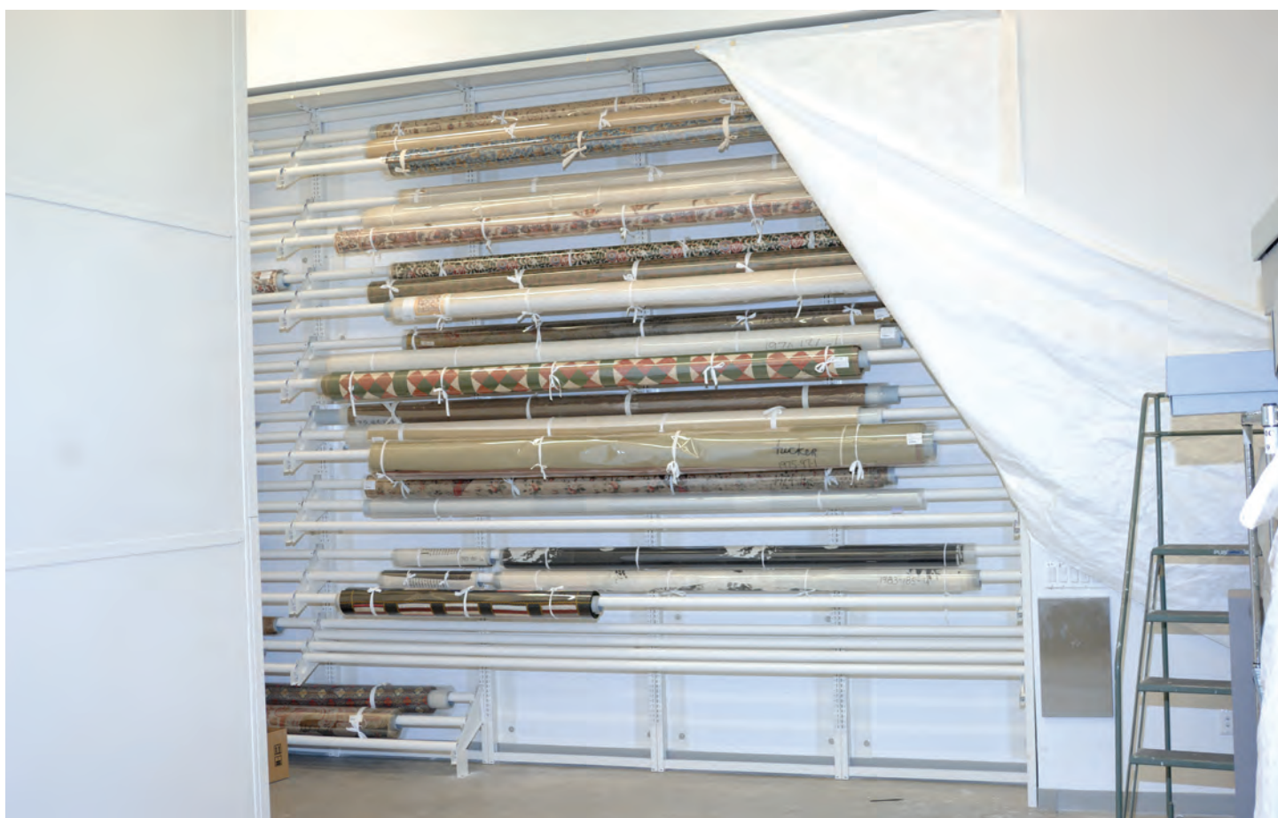
Figure 8. Bracket system to hold long rolled textiles.
