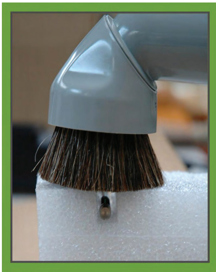
Figure 8. Setup 2 – Measuring shear (parallel or tangential) forces (i.e. air flow) using the anemometer. Measurements were taken using several vacuum attachments, including the upholstery brush, seen here.
